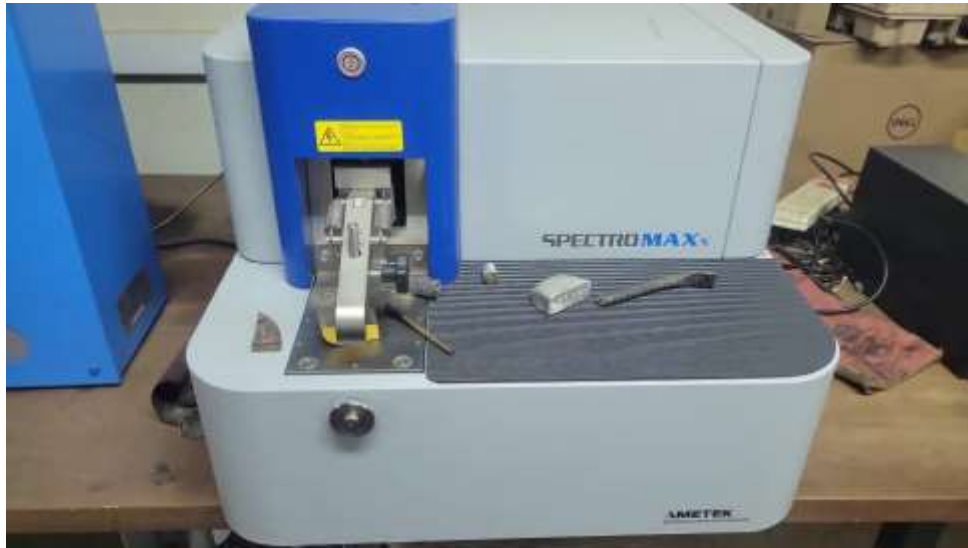
Figure 3.2: Spectro max used to determine the chemical composition of the welds
