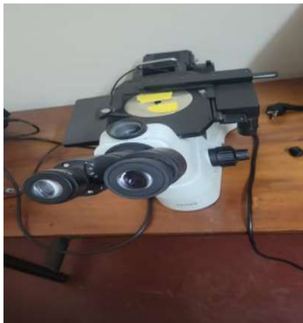
Figure 3.6: Optical Microscope used to analyze the grain structure of the welds
