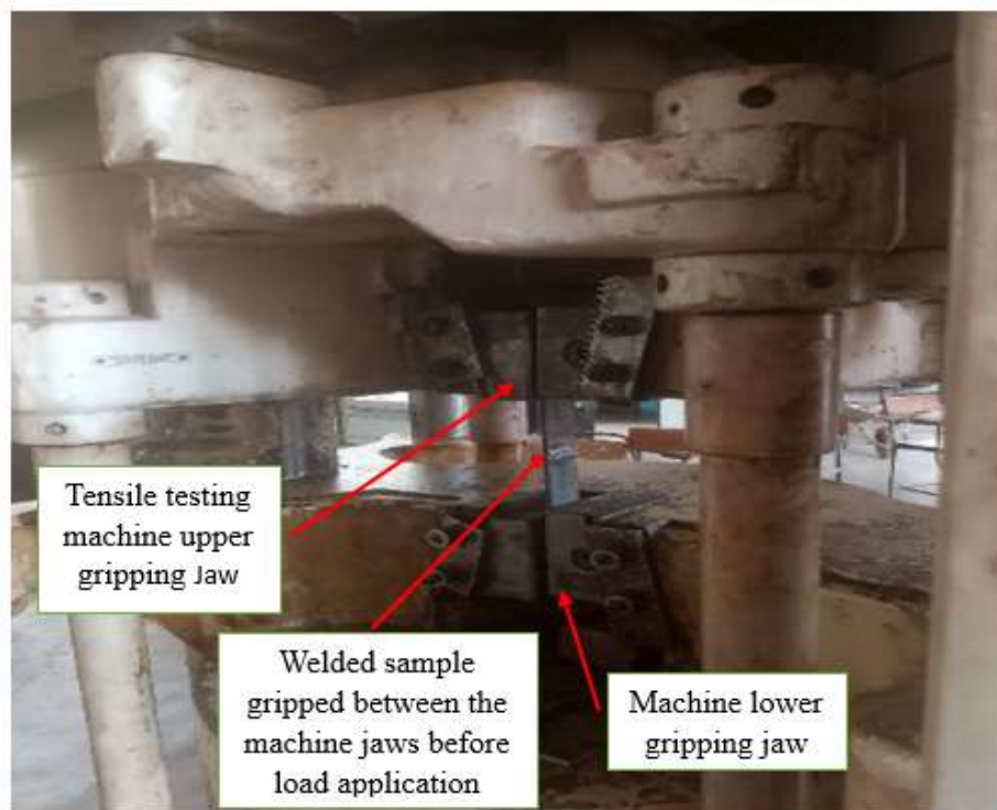
Figure 3.5: Specimens mounted on Denison tensile testing machine
