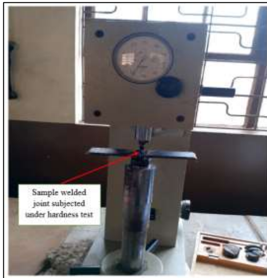
Figure 3. 4: Specimen under evaluation for hardness
