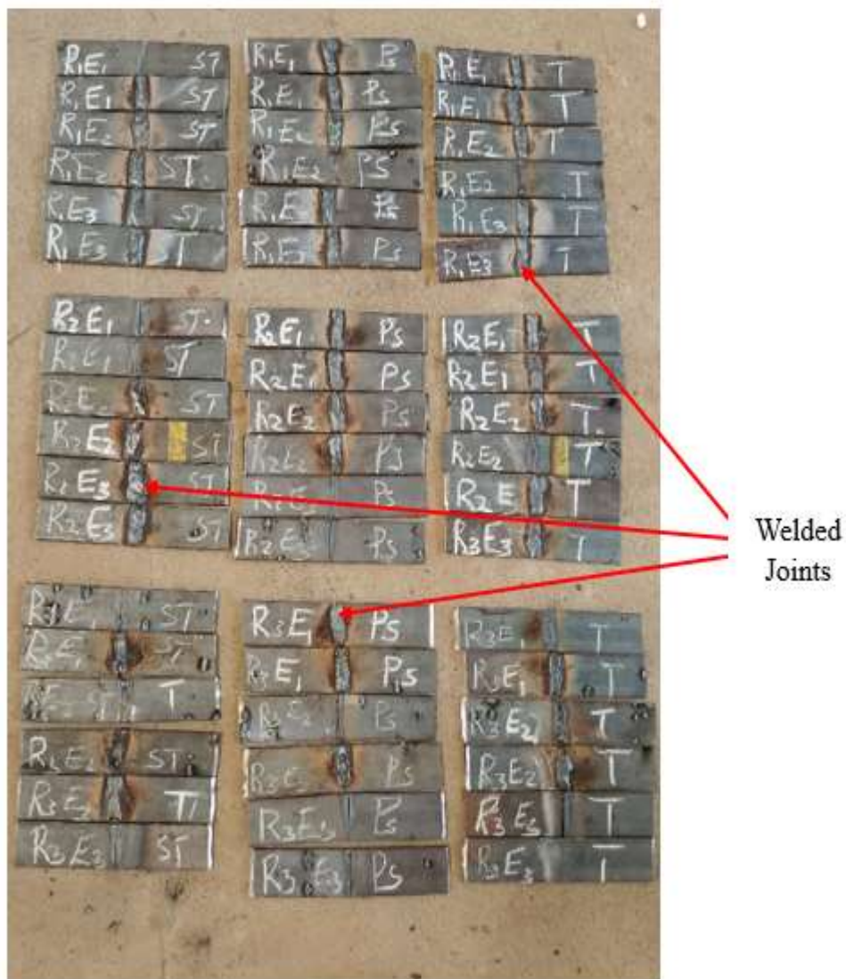
Figure 3.3: Specimens welded in a flat position with a single pass
