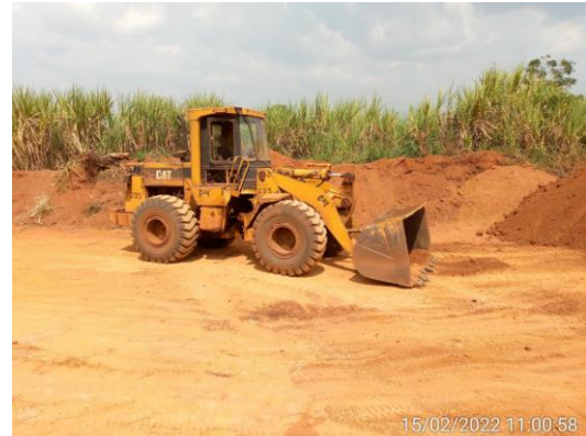
Figure A. 2: CAT 950H Front End Loader.
