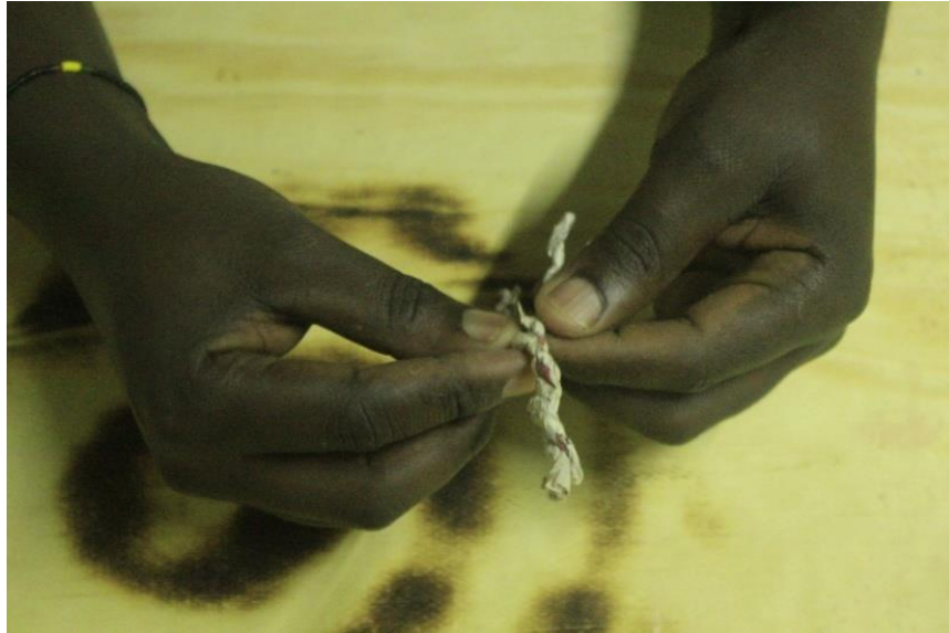
Figure 57: The process of twisting and rolling two rolled paper to form a paper rope.
