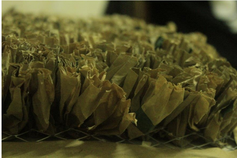
Figure 64: The process of pressing cut paper pieces into a wire mesh and then weaved through the wire.
