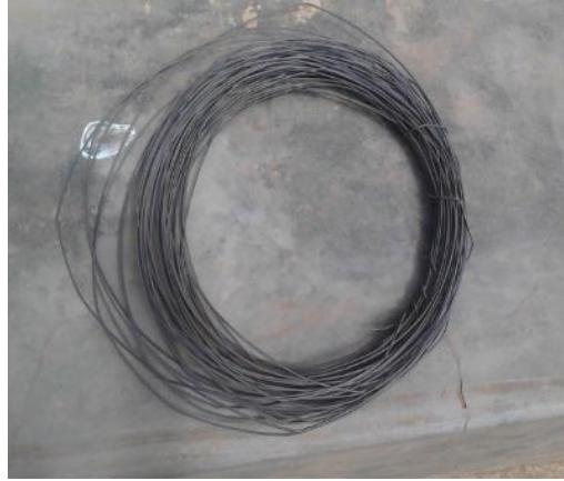
Figure 30: Binding Wire Source: Photograph taken by researcher
