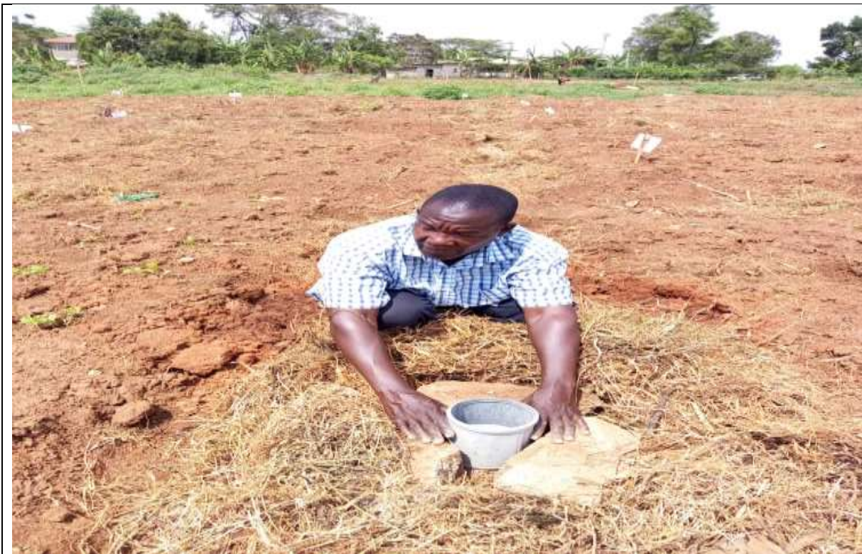
Plate 5: Rain gauge in the experimental lay out to collect data on amount of rainfall
