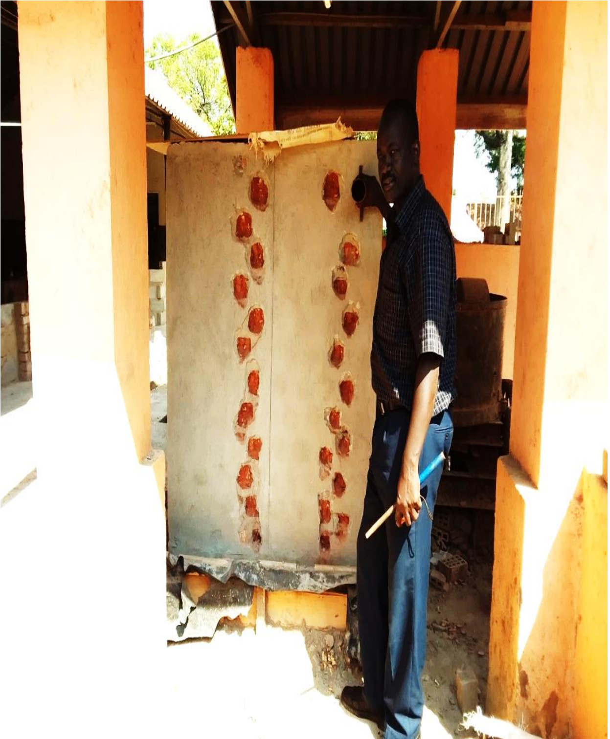
Figure A3.14: showing the researcher comparing samples for m.c examination at different heights on the vertical face of one of the internal models, at Kyambogo University Soil Laboratory
