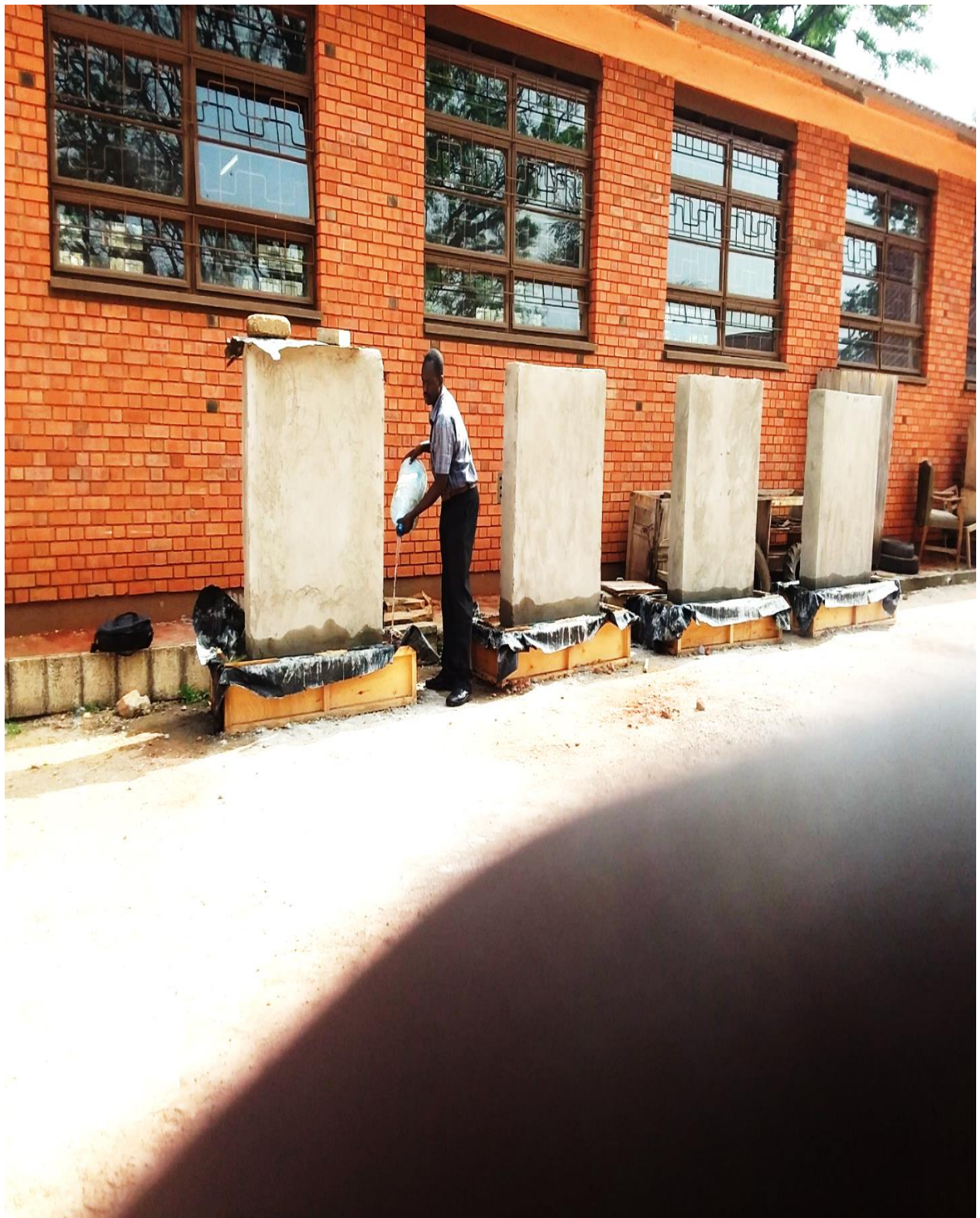
Figure A3.10: showing the researcher feeding the experimental models with water, at Kyambogo University Soil Laboratory
