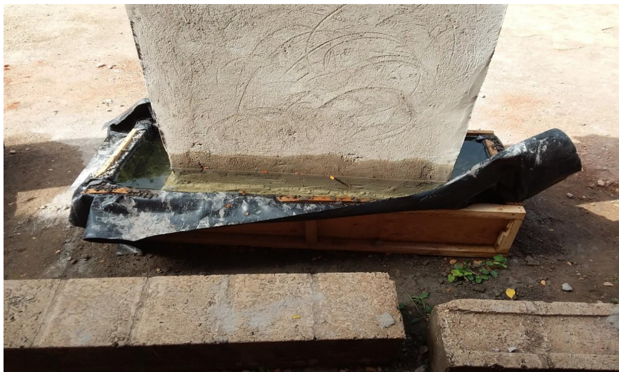
Figure A3.6: showing moisture rise through the researcher's experimental model 2 simulating a masonry wall, at Kyambogo University Soil Laboratory
