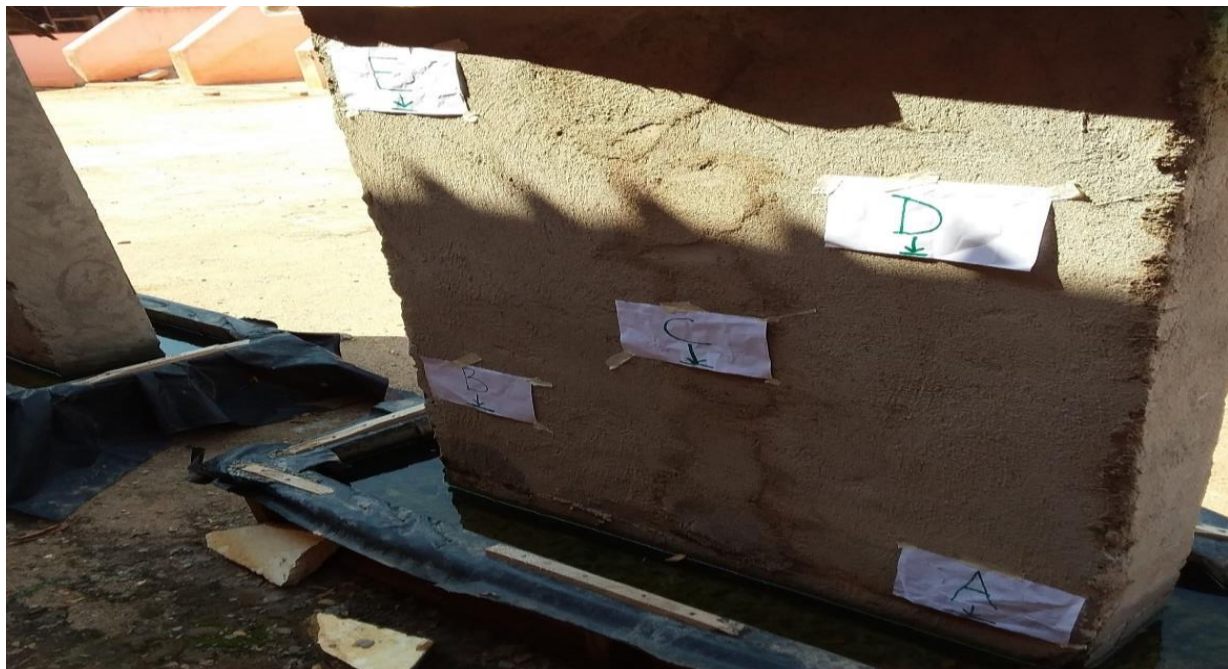
Figure 3.8: Selected points on the face of one of the models, with water
