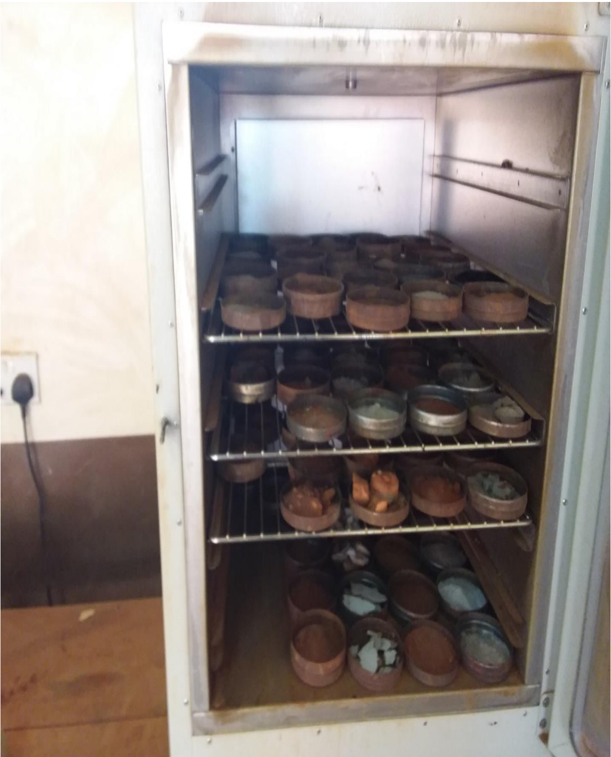
Figure A3.15: showing the researcher examining m.c on the samples in an oven, at Kyambogo University Soil Laboratory
