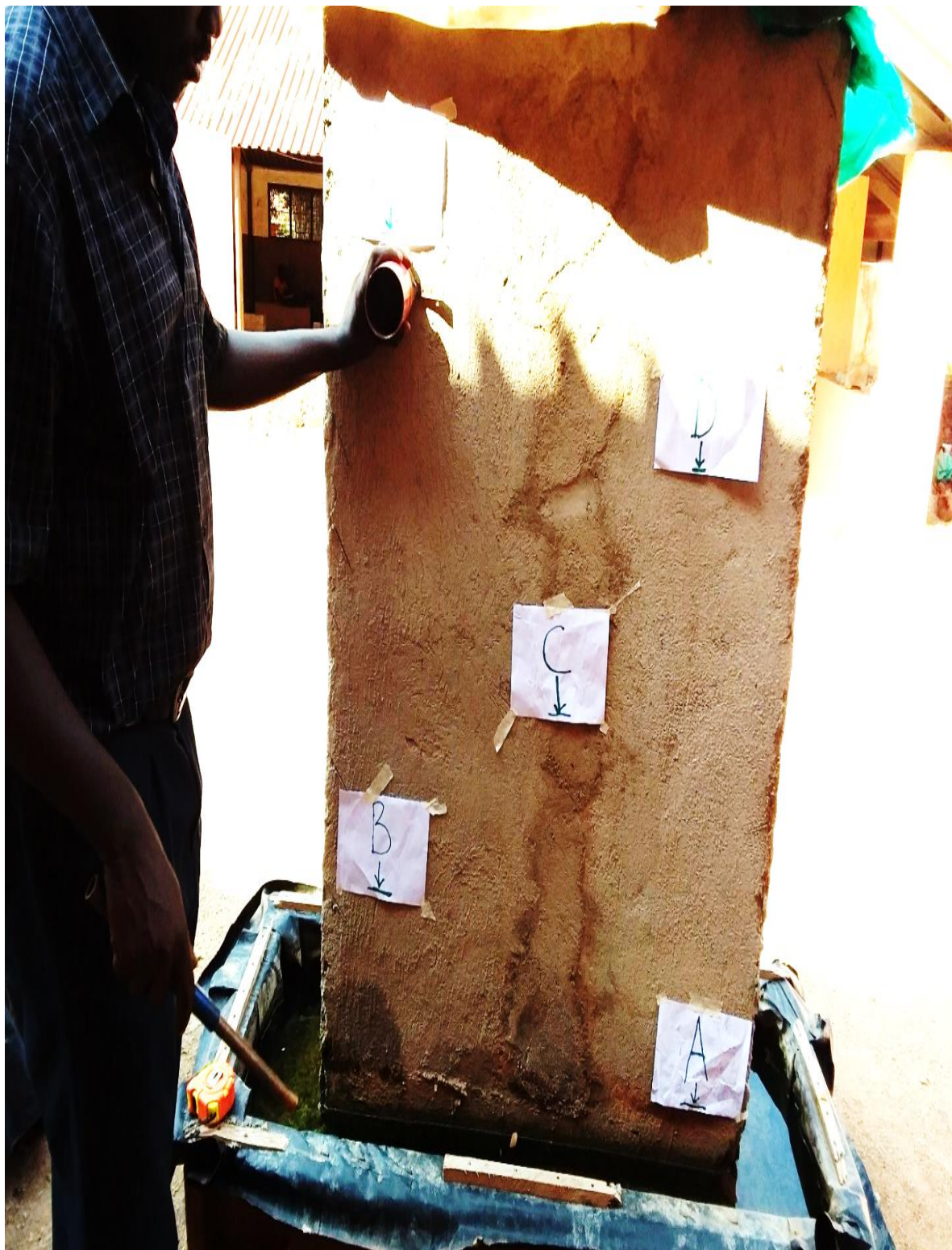
Figure A3.13: showing the researcher picking samples for m.c examination at different heights on the vertical face of one of the models, at Kyambogo University Soil Laboratory
