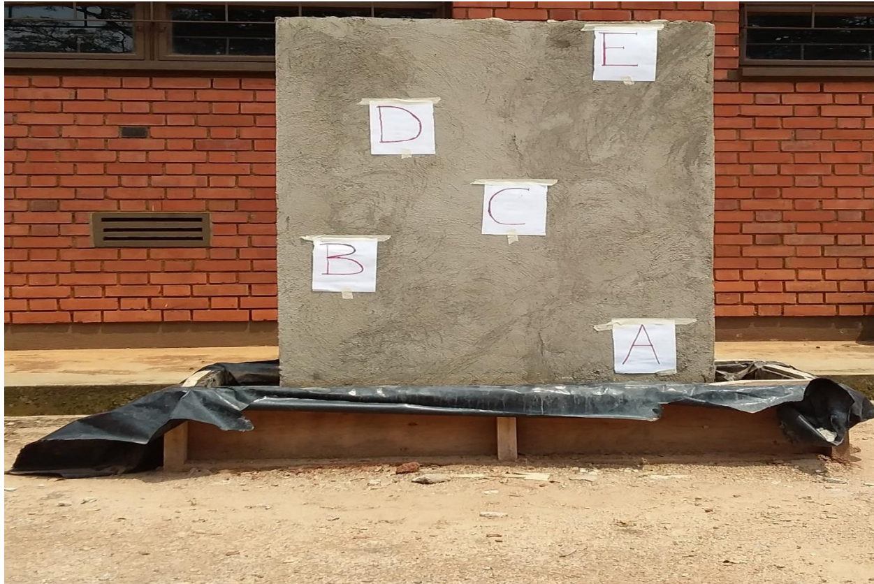
Figure 4.1: Sample plaster taken from different spots on the face of model 5 outdoor 1 cement sand ratio 1:3
