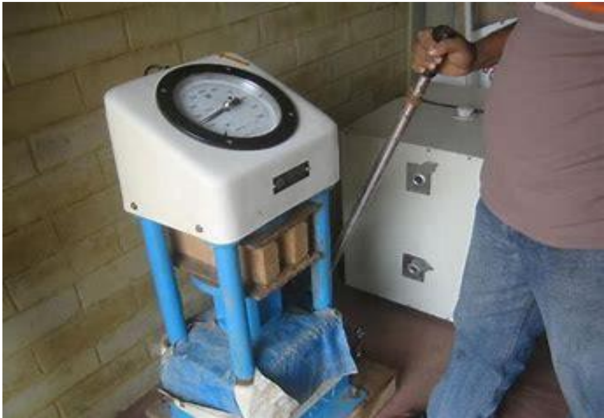
Figure 3.2: Compressive Strength Measuring Machine
