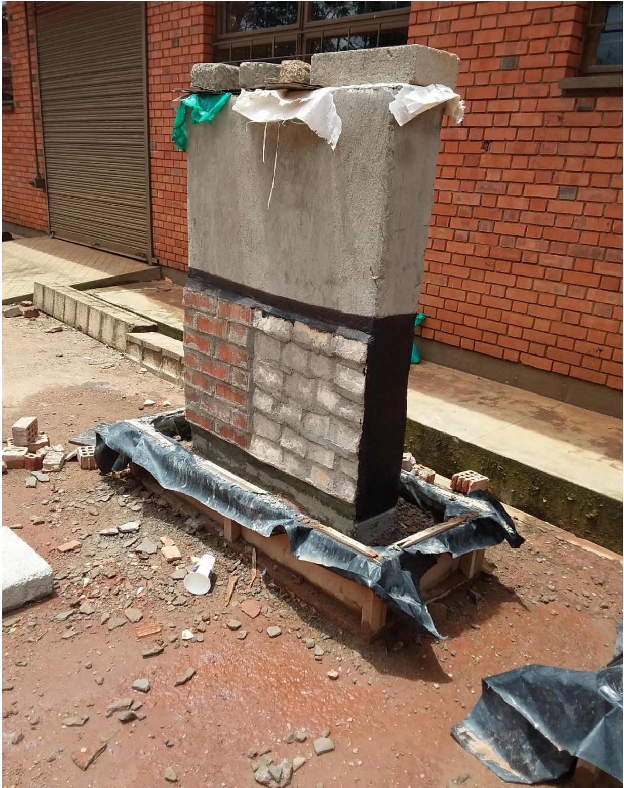
Figure A3.16: showing the different materials being examined for solution to moisture rise in masonry walls, at Kyambogo University Soil Laboratory
