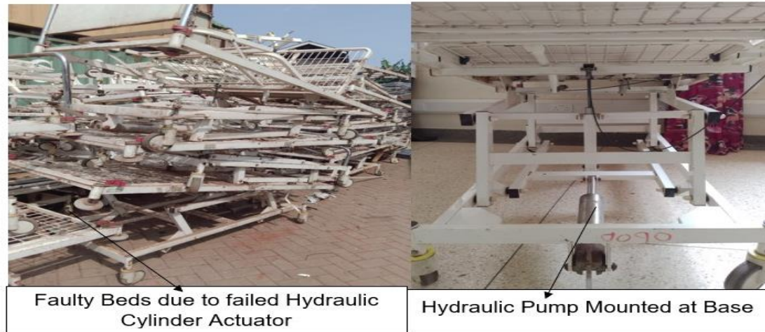
Figure 1. 1: Faulty beds due to faulty hydraulic cylinder actuator mounted at base
