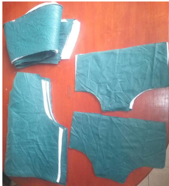
Figure 64 The different parts of the twin baby carrier cut and ready to be sewn together.
