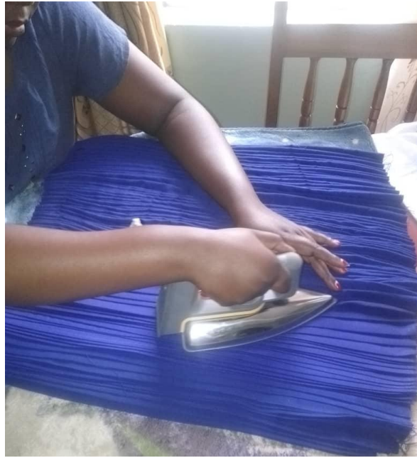
Figure 49 The researcher ironing the pin tucks after sewing so that they can be flat
