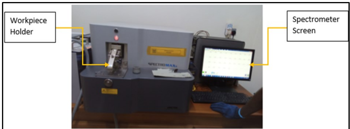
Figure 3.8: Shows the mass spectrometer machine (Taken with permission from Roofing Rolling Ltd.)
