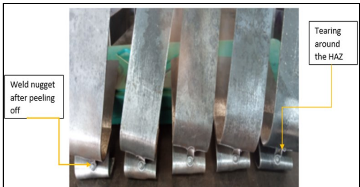
Figure 4.7: Test pieces after the peel test
