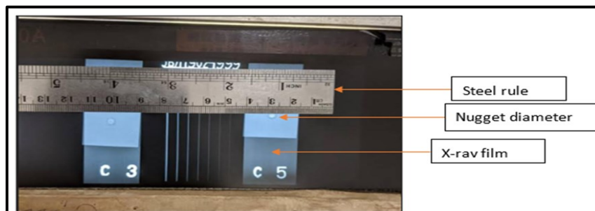
Figure 3.12: Measurement of the nugget diameter from the X-ray film
