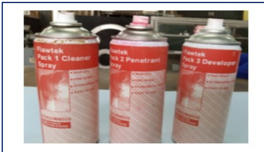
Figure 3.10: A set of dye penetrant that was used in dye penetrant method.
