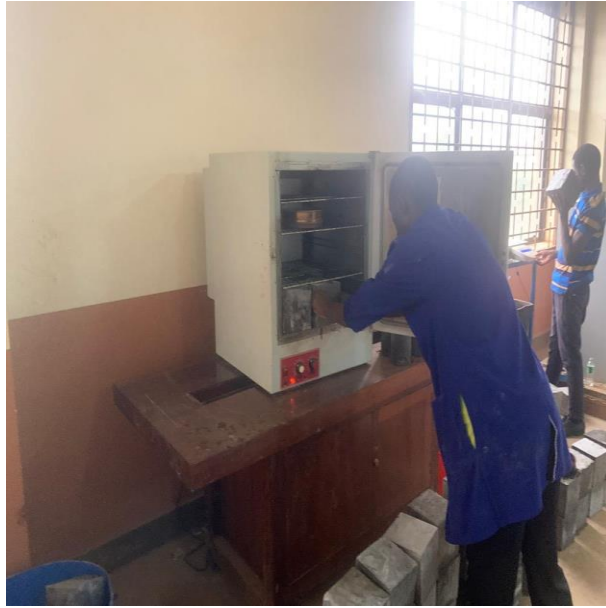
Figure 3.11 Oven-drying concrete cubes
