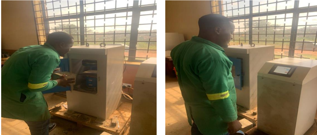
(e) Placing concrete mould on UTM's loading platform (f) Reading compressive load from UTM screen
