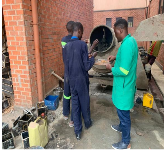
Figure 3.5 Batching and fibre incorporation
