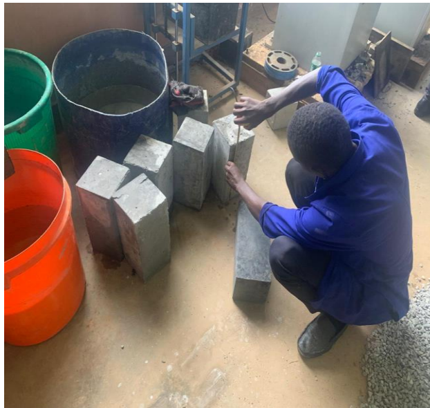
Figure 3.9 Measuring concrete prism length
