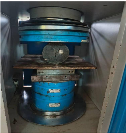
(h) Exerting load onto concrete cylinder
