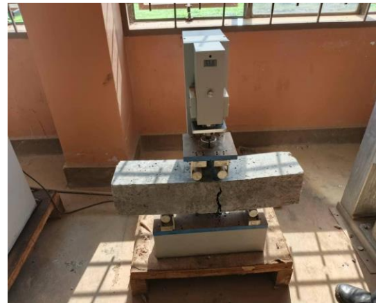
(j) 2-point loading on concrete beam
