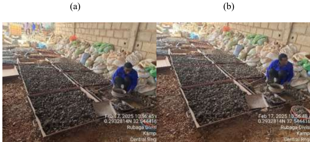
Figure 3.2: Air drying and sieving clay samples at Teclab in nalukolongo
