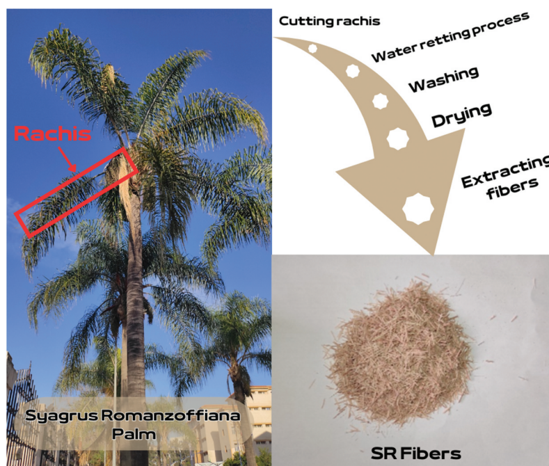
Figure 1. Process of extracting fibers from Syagrus palm rachis waste.
