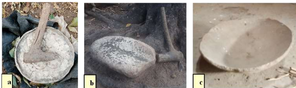
Figure 4.37: A mallet, a saucepan and polythene for mixing (a) A grinding stone (b), and a moulding base(c)
