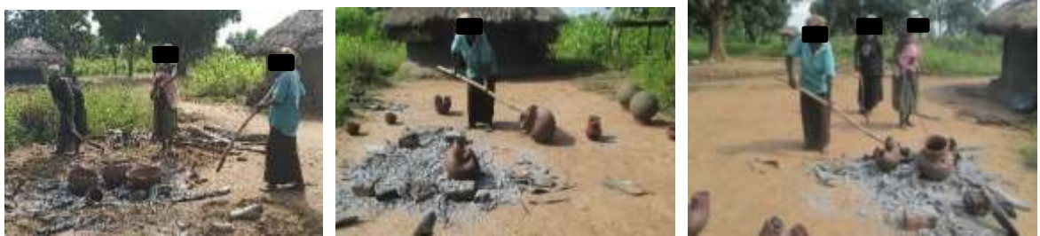
Figure 4.49: Removing the fired pots using long sticks.
