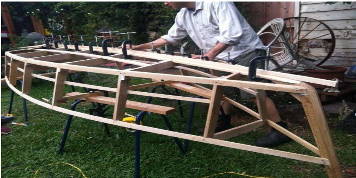
Figure 12: Frames and other structural members before planking
