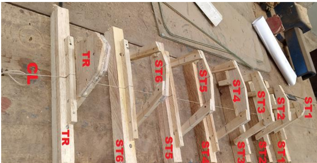
Frames assembled on a building jig Source: Primary Data 2022
