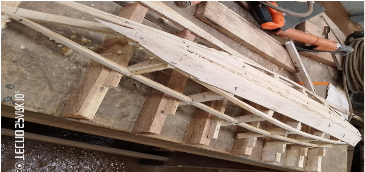
Scale model (prototype) at planking stage
