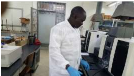
Water analysis process for the heavy metals using Atomic Absorption Spectrum at Makerere – Chemical Laboratory.
