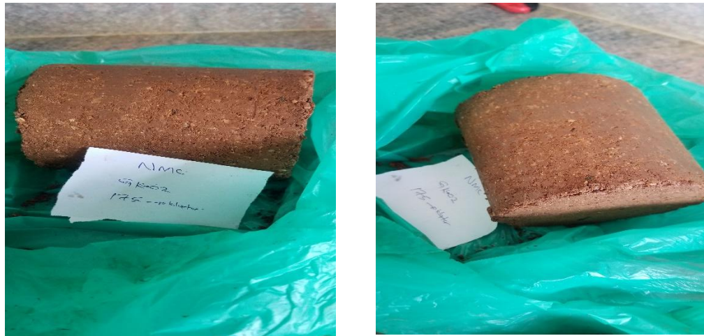
Figure G. 11: Remolded samples/compacted specimen for double oedometer
