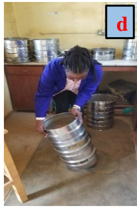
Figure G. 5: a. Soaked samples in preparation for wet sieving, b. Wet sieving with a sieve of 0.075 mm aperture sieve, c. BS sieves with decreasing aperture that was used for dry sieving, d. Dry sieving, e, and f. Weighing the material retained on each sieve
