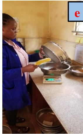
Figure G. 5: a. Soaked samples in preparation for wet sieving, b. Wet sieving with a sieve of 0.075 mm aperture sieve, c. BS sieves with decreasing aperture that was used for dry sieving, d. Dry sieving, e, and f. Weighing the material retained on each sieve
