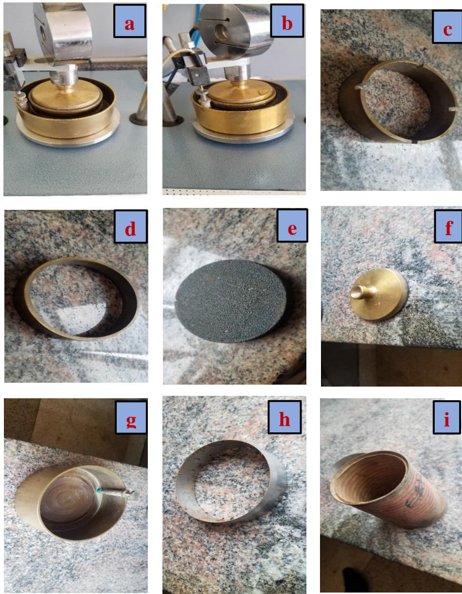
Figure G. 12: a. Unsaturated loaded sample, b. Saturated loaded sample, c. d. e. Porous Stone f. Loading Pad g. h. Cutting Ring, i. Moisture tin.
