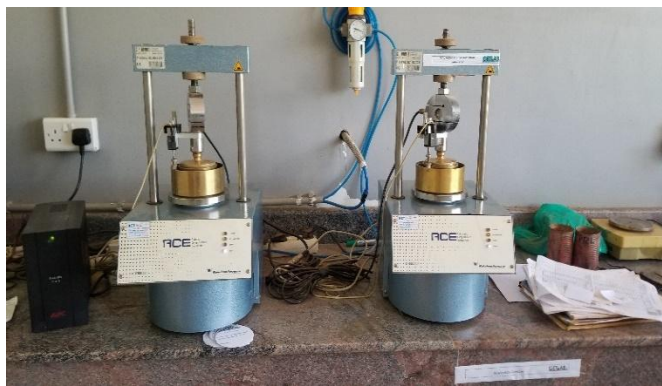
Figure G. 14: Loaded samples for double oedometer test at NMC, one saturated and the other unsaturated
