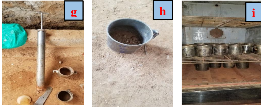
Figure G. 10: a. Preparation of the sample by sieving through the 20mm and 5mm aperture sieve, b. Measuring cylinder used to track the amount of water added to the sample, c. Weighing the sample to be used at each point, d. Oiling the mould to avoid sticking of the sample to the mould, e&f. compaction in layers 5 layers- 27 blows on each layer, g. 4.5kg rammer, h. Moisture tin, i. Oven drying moistures for 24 hours.
