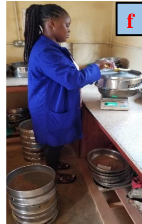
Figure G. 5: a. Soaked samples in preparation for wet sieving, b. Wet sieving with a sieve of 0.075 mm aperture sieve, c. BS sieves with decreasing aperture that was used for dry sieving, d. Dry sieving, e, and f. Weighing the material retained on each sieve
