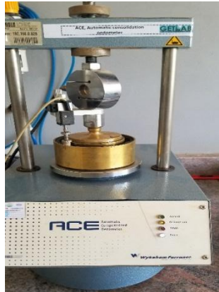
Figure G. 13: Loaded sample in the conventional oedometer or the single oedometer test
