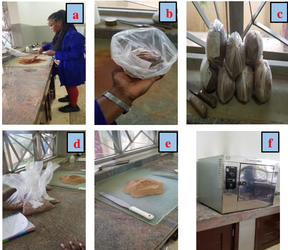
Figure G. 7: a. Preparation of the samples, b. One of the soil samples kept in an air-tight bag and soaked for 24 hours after which the experiment was conducted using the cone penetrometer method, c. Samples soaked for 24 hours, e. Oven
