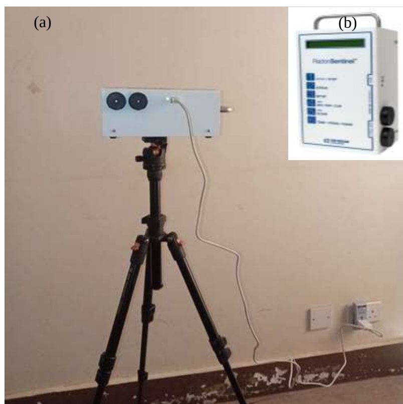
Figure 3.2: (a) Set-up of Radon Sentinel Monitor (model 1030), and (b) Radon sentinel Detector.
