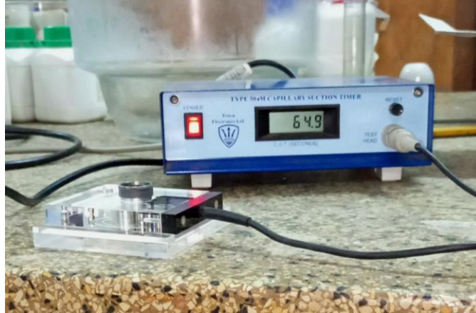
Figure 3-5: A capillary suction timer during the measurement the dewaterability rate of a sample.
