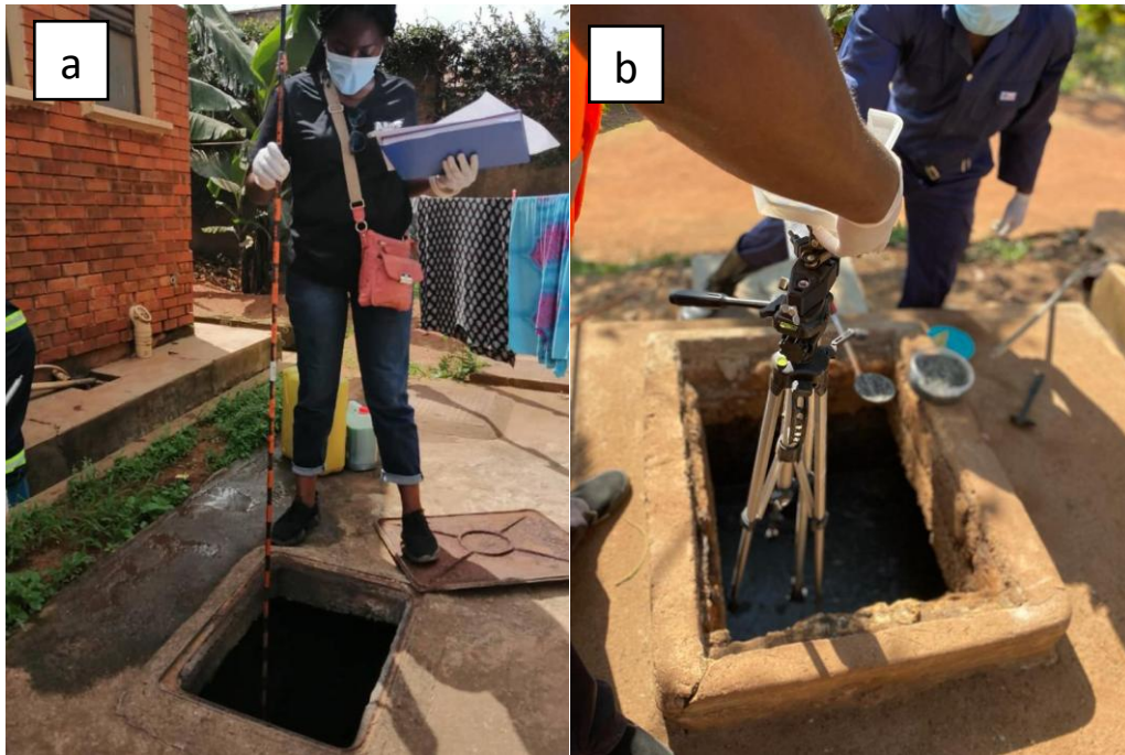
Figure 3- 2: Measurement of depth of both FS and FSS using L-stick (a) and (b) surface area of the septic tank using the Volasor.
