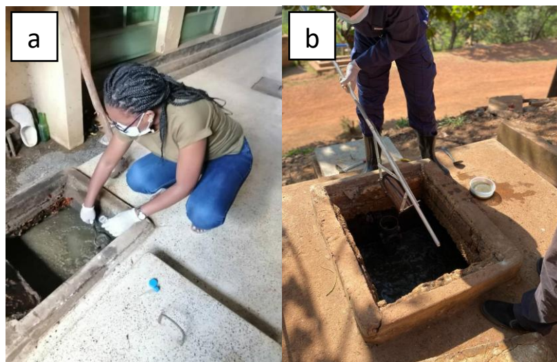
Figure 3- 4: Sampling of FSS from the surface of septic tank using a scooping spoon (a) and (b)FS using improvised long-handled container.
