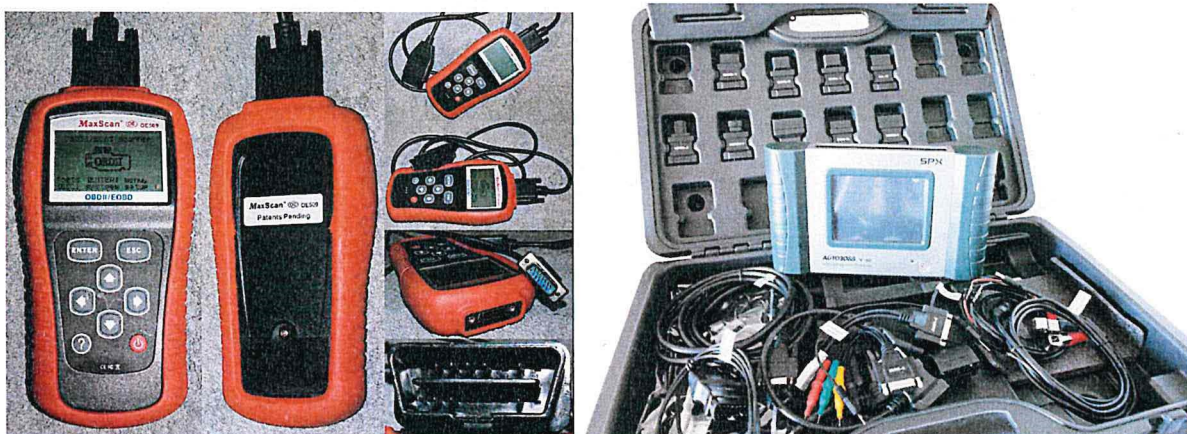
Figure 10: Various angles of a "Max Scan OE509" and a Multi-brand vehicle diagnostics hand held system Auto Boss V-30
