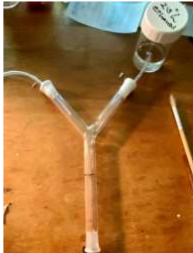
Figure 6: Y-tube olfactometer used to study BCTB response towards different ethanol concentrations.
