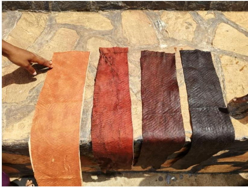
Figure 32: Sample shades of barkcloth after dying in clay water for different minutes. The darkest was dyed for longer than the rest.
