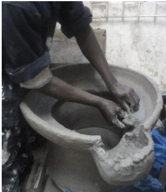
Figure 79: Modeling the lower section of water fountain. Source: Researcher, 2020.
