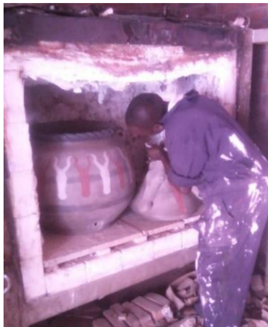
Figure 74: Loading green ware in an electric kiln for firing. Source: Researcher, 2020.
