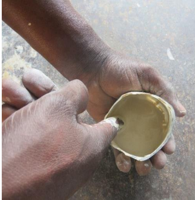
Figure 62: kaolin mixed with secondary clay slip to enhance plasticity. Source: Researcher, 2020.
