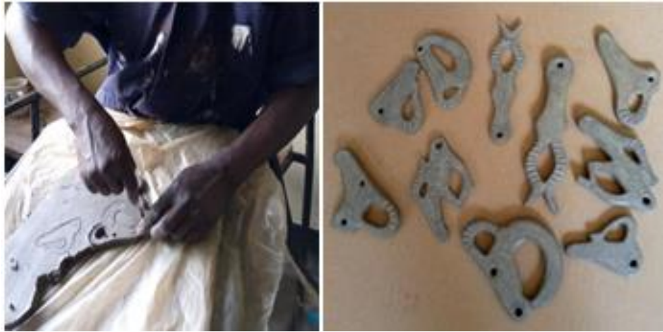
Figure 113: Cutting out shapes of key holders from clay slab. Source: Researcher, 2020.
