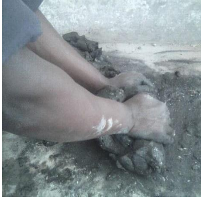
Figure 67: Ceramics stains being wedged and kneaded with clay ready for use. Source: Researcher, 2020.
