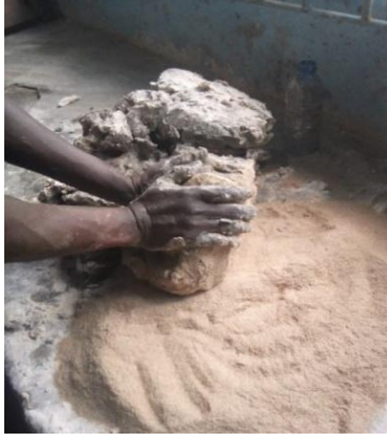
Figure 64: Wedging and kneading clay with sawdust ready for use. Source: Researcher, 2020.
