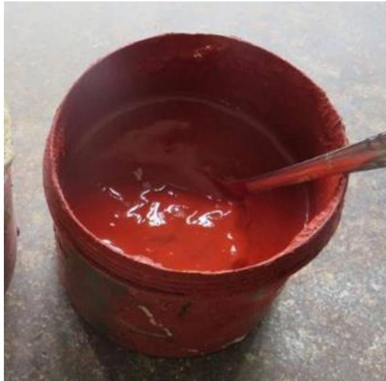
Figure 66: Ceramics red oxide mixed in water and clay slip to enhance plasticity Source: Researcher, 2020.
