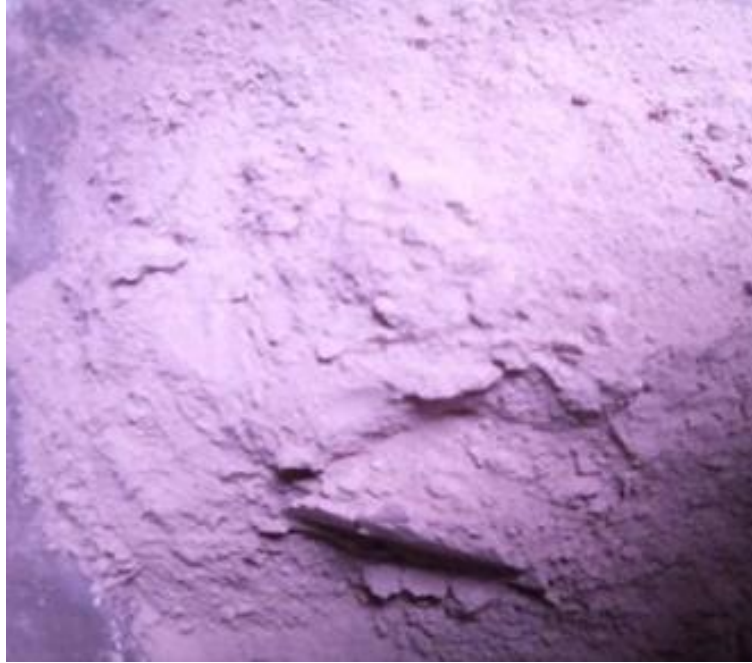
Figure 63: Crushed and sieved grog. Source: Researcher, 2020.
