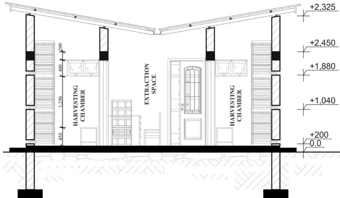
Figure 4.8.51 Cross-section X through the RBH captures the lintels.
