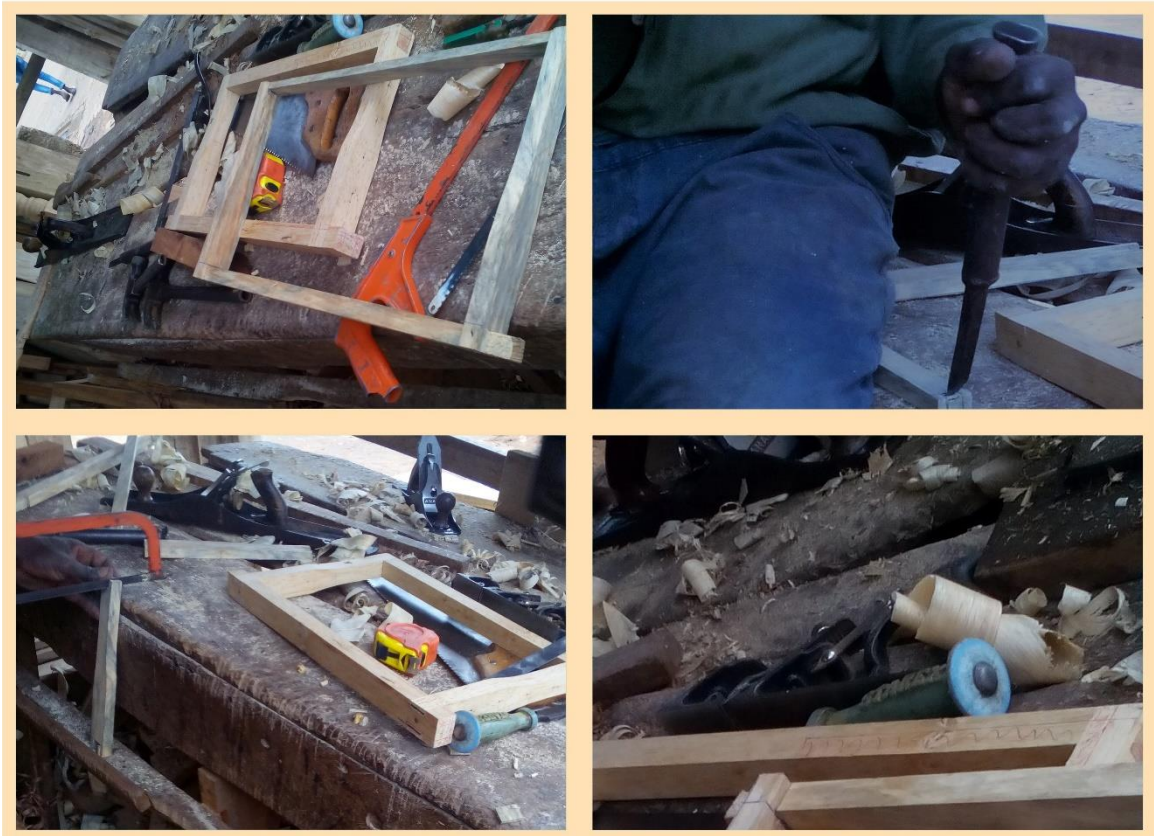
Figure 4.8.46 The Langstroth frame being constructed by a local carpenter under the supervision of the researcher to test the ability of the carpenter to capture it precisely
