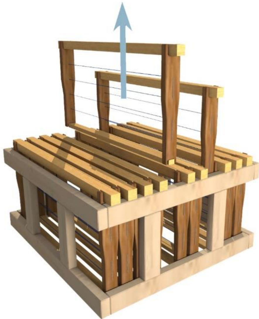
Figure 4.8.62 The crate laden with the 12 frames to be installed in the RBH Illustration by researcher, 2020
