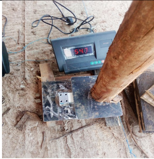
Load cell under prop and indicator
