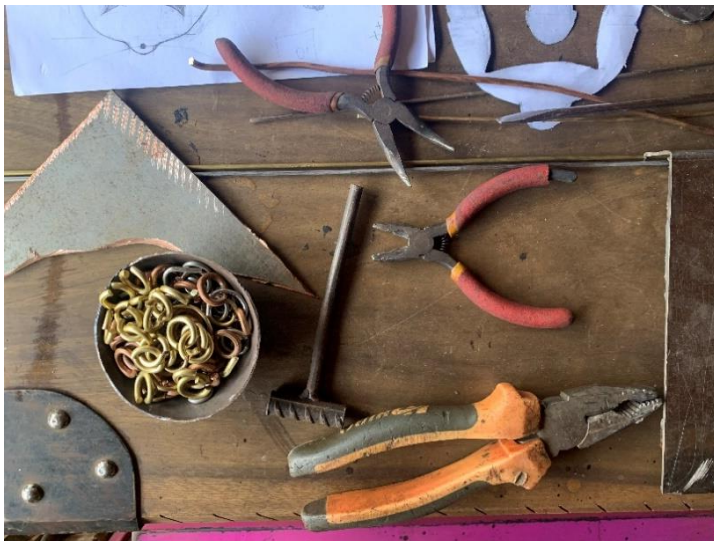
Figure 17: Part of the design process which involved cutting out the respective designs from aluminium, copper and brass plates alongside some of the tools used namely: pair of pliers and a hammer.
