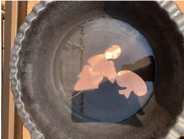
Figure 22: Brass designs immersed in water after sanding aimed at cooling their temperature down alongside cut out designs displayed to pave way for buffing, doming and punching. Source: Photograph taken by researcher
