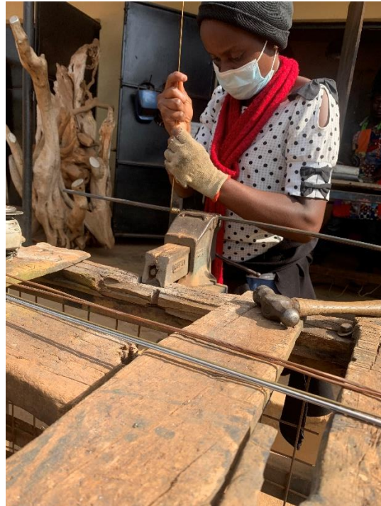
Figure 23: The researcher curving copper, aluminium and brass rods into chains Source: Photograph taken by researcher
