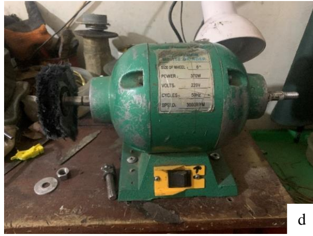
Figure 18: Images a, b, c and d showing a saw frame, a drill, drill bit, tripoli and a bench grinder respectively
