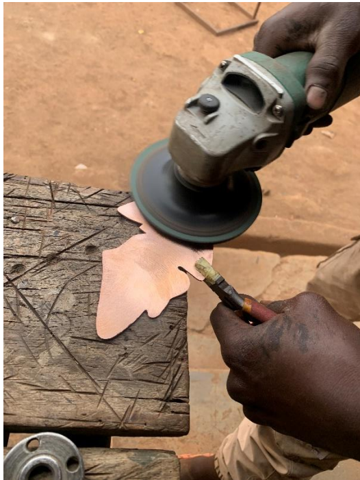
Figure 21: The researcher using a grinding machine to clean brass and a cutting machine to cut out the respective designs
