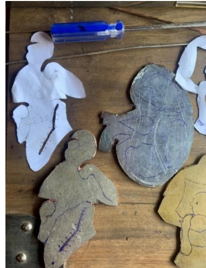
Figure 17: Part of the design process which involved cutting out the respective designs from aluminium, copper and brass plates alongside some of the tools used namely: pair of pliers and a hammer.
