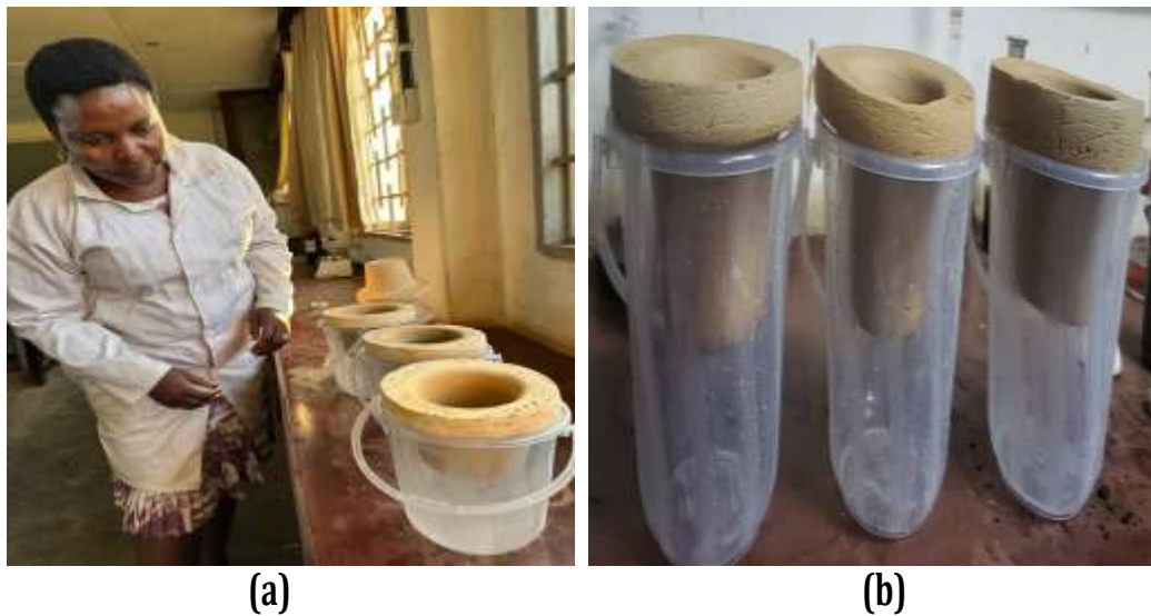
Figure 3.5: Experimental Set up of Lead Removal
