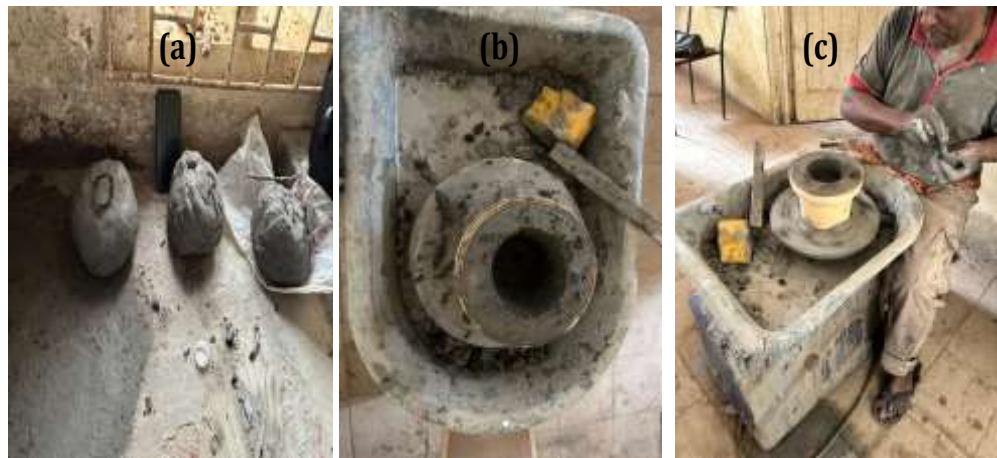
Figure 3.3: Clay filter preparation process
