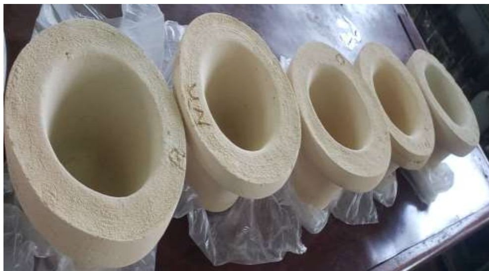
Figure 3.4: AgNPs impregnated clay filter Models
