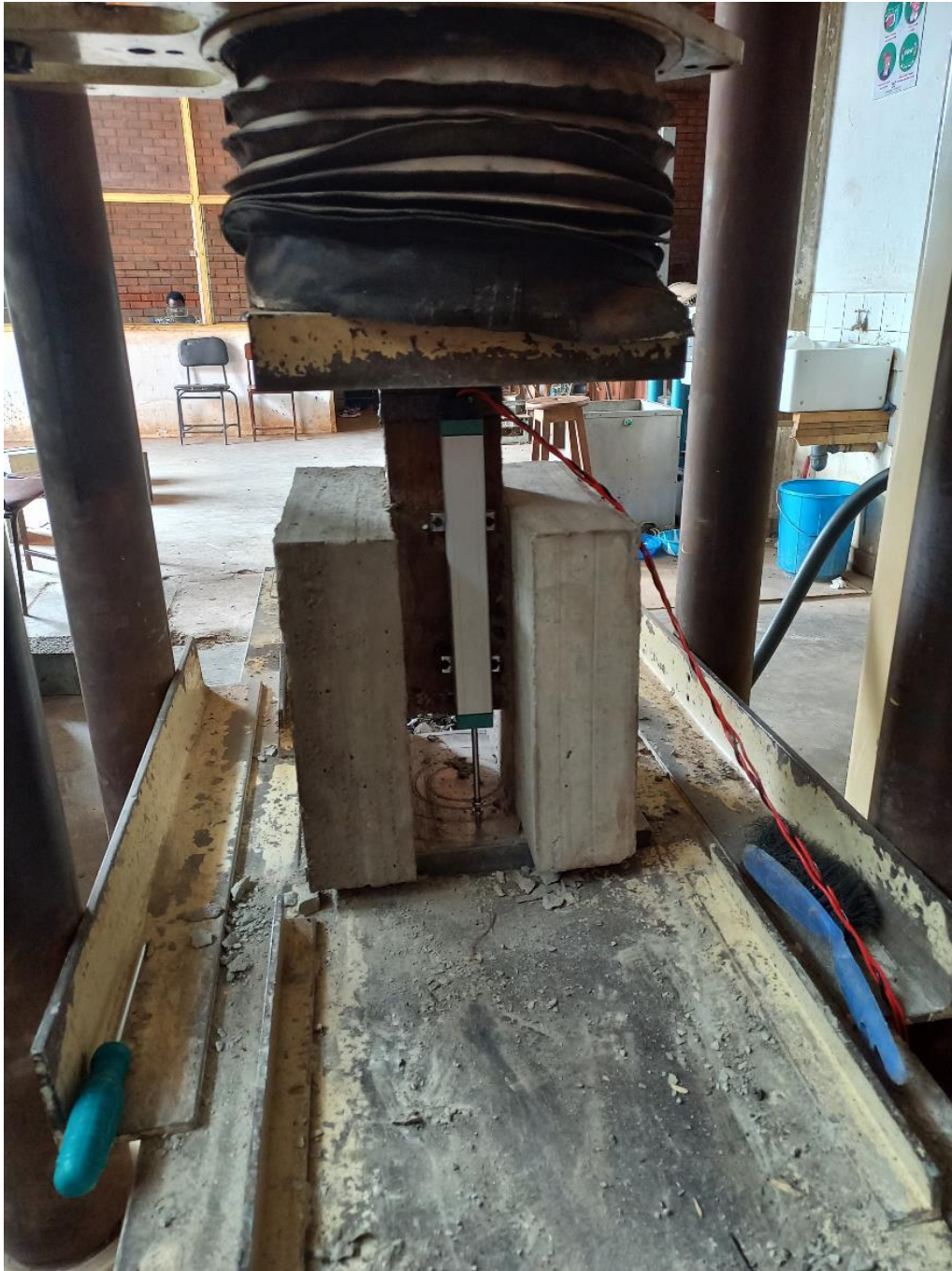
Figure 3.12 The setup of the push out test experiment before testing
