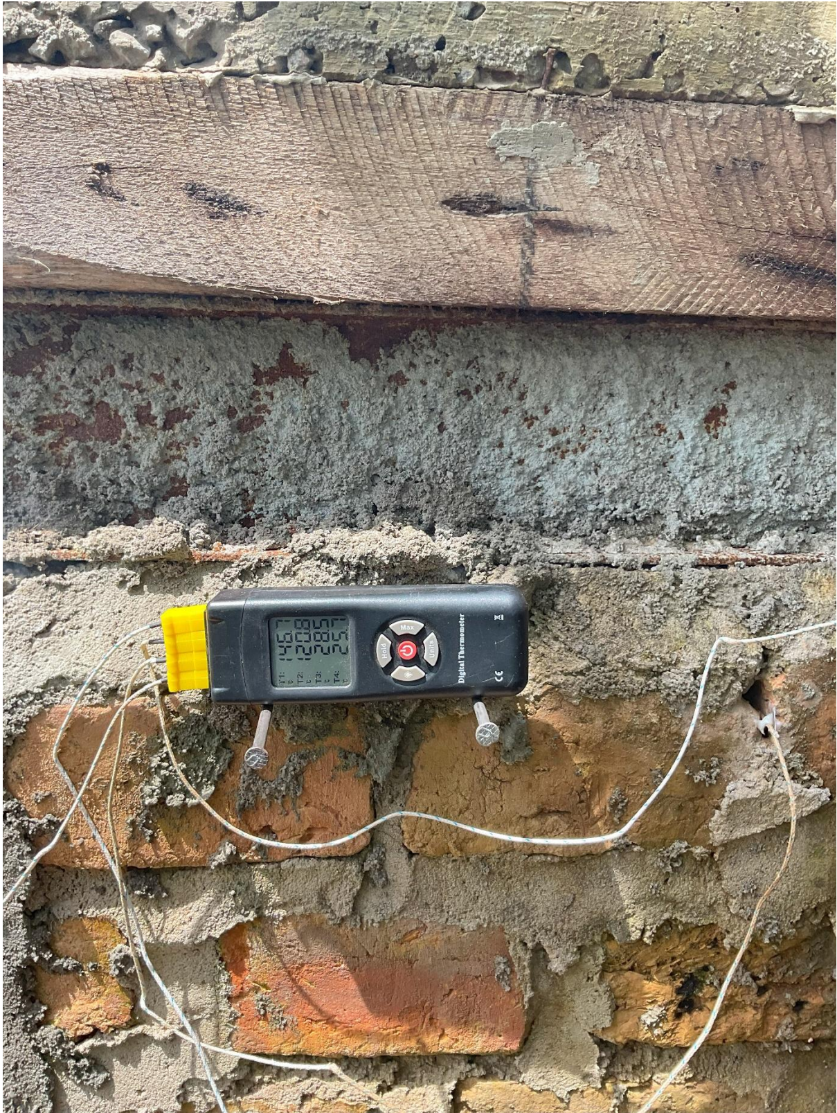
Figure D.8: Digital thermometer connected to K-thermocouples for taking temperature readings
