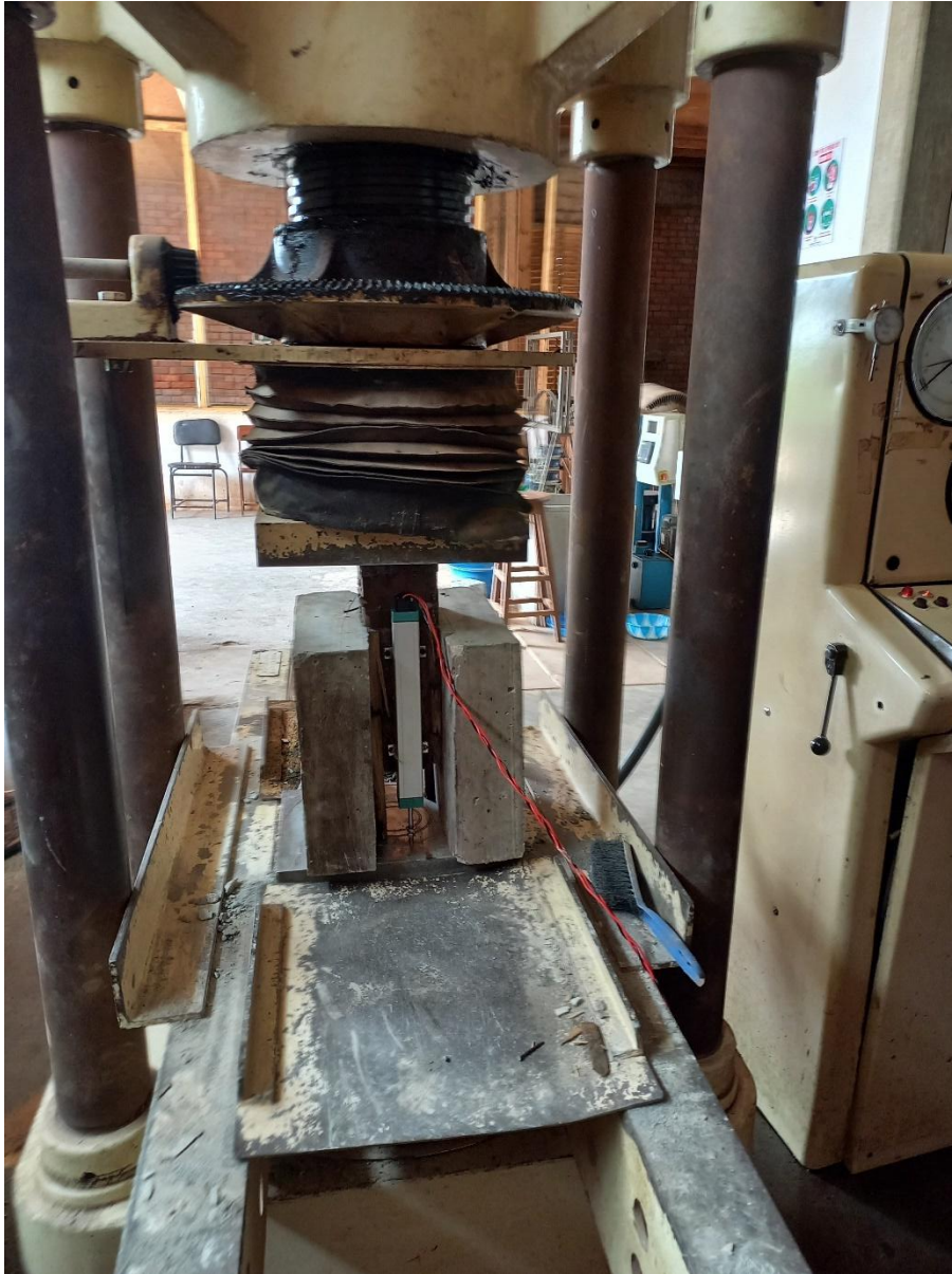
Figure D.3: Setting Universal testing machine (UTM) before testing, loaded with push out sample which was mounted with a Linear variable displacement transformer (LVDT) for measuring slip
