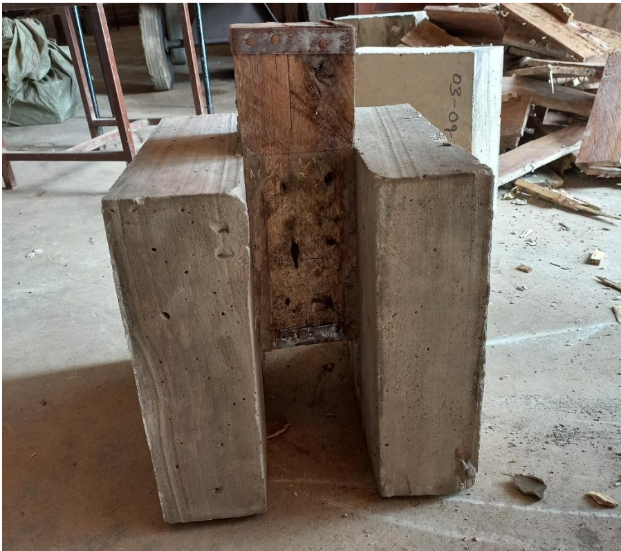
Figure 3.11: A physical pushout test specimen ready for testing.
