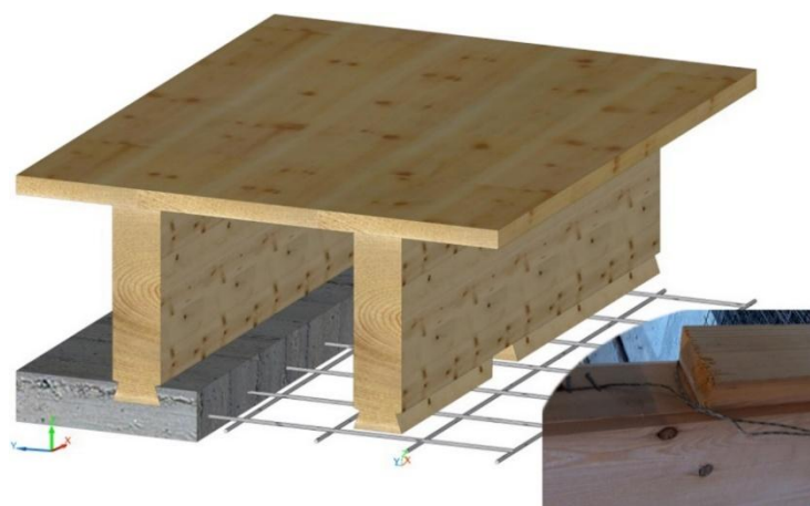
Figure 2.10 The schematic illustration of the novel Timber Concrete Composite system (Meena, et al. , 2014)
