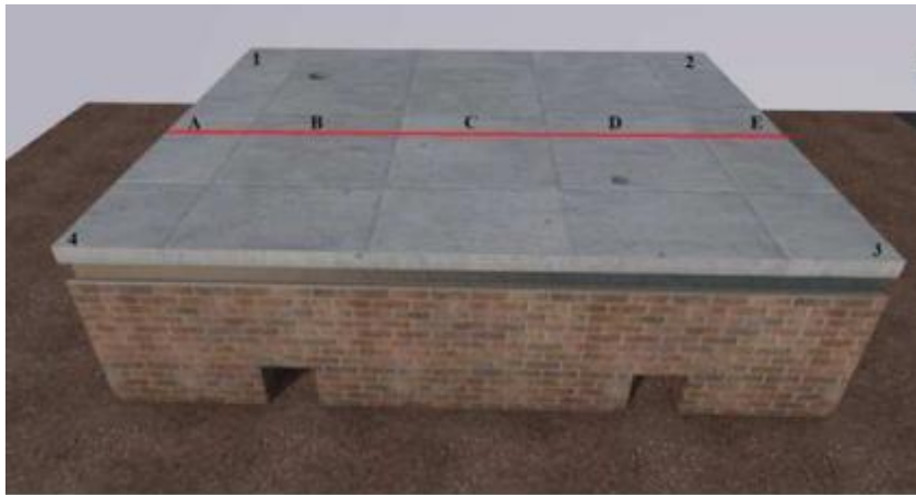
Figure 3.3 shows the location of the linear variable transducers on the slab to detect deflection
