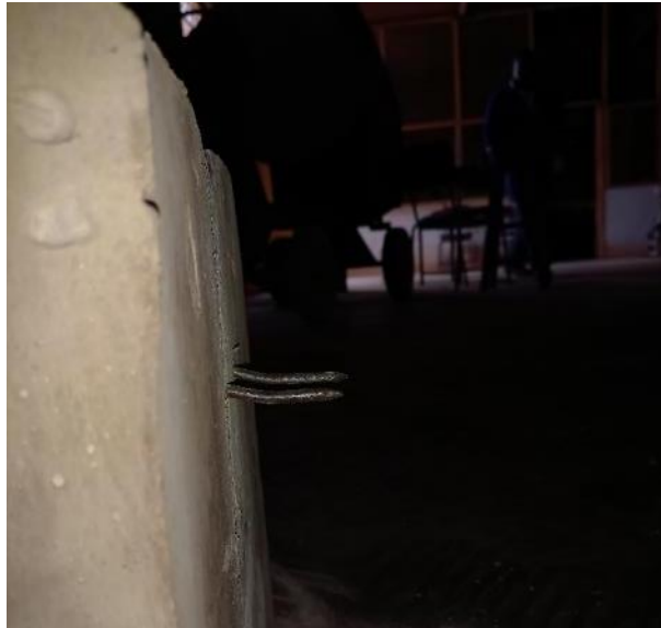
Figure 4.36: shows Plastic deformation of the nails and concrete showed no sign of failure
