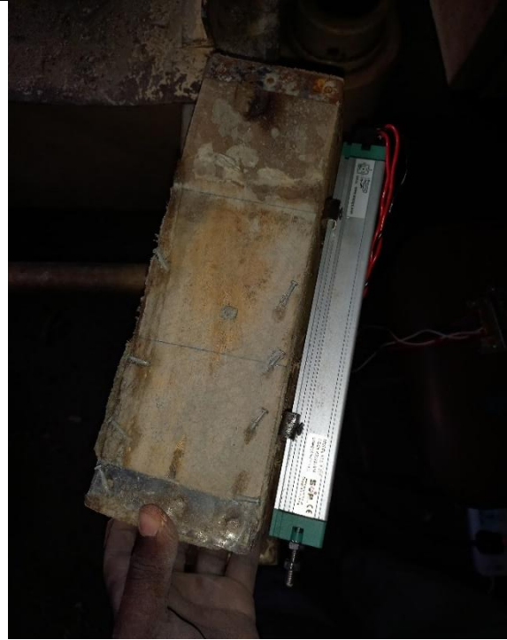
Figure 4.41: Timber that was attached to one of the Expanded Metal lathe (Mesh) samples. the bent nails were used to connect the Expanded Metal lathe (Mesh) to the timber
