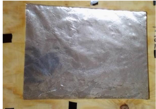
iv Gel spread on the mould
