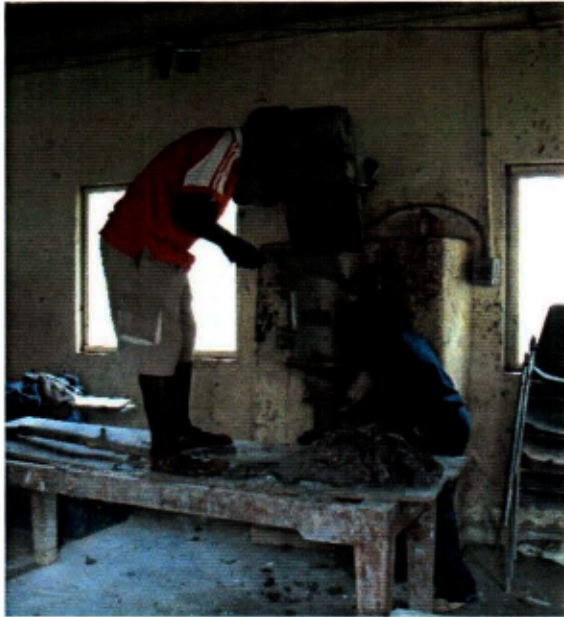
Plate XXI: Pug-mill machine. Used for preparing clay for ceramics (2010)
