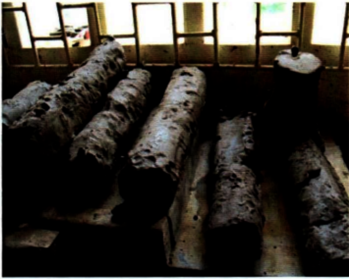
Plate XXII: Prepared Clay using Pug-mill, the action of reconstituting clay by Passing it through a pug mill which is a form of mincing machine Source: Ceramic Department Kyambogo University
