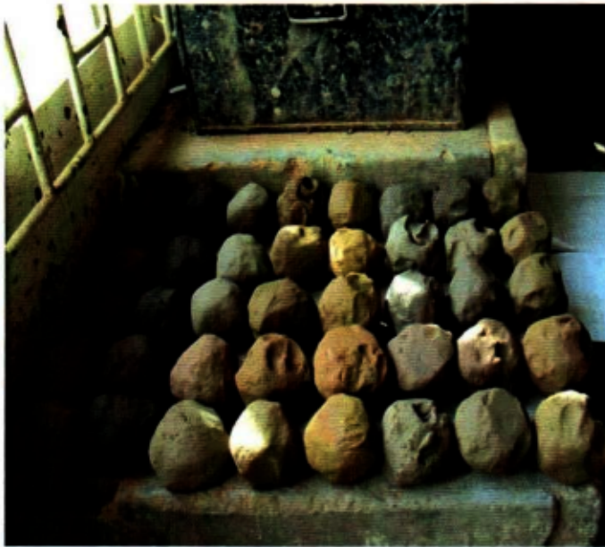
Plate XXIII: Different clay bodies mixed with parts of grog, sand and kaolin.
