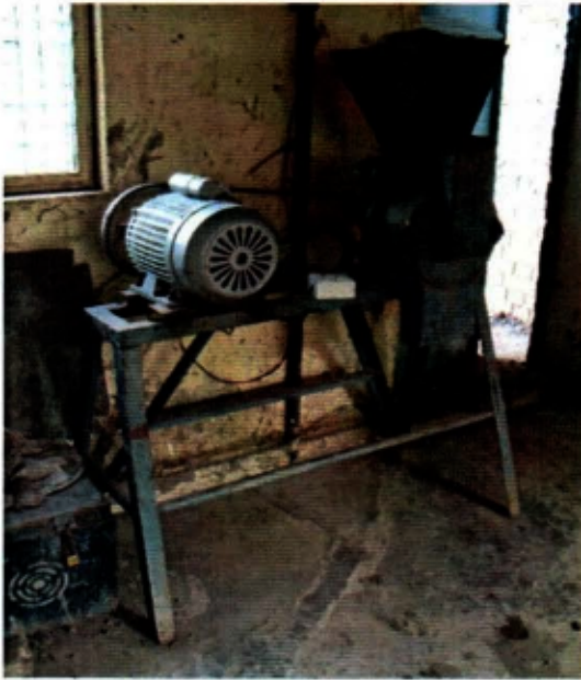
Plate.XVI: Clay grinding mill. Source: Ceramic Department Kyambogo University
