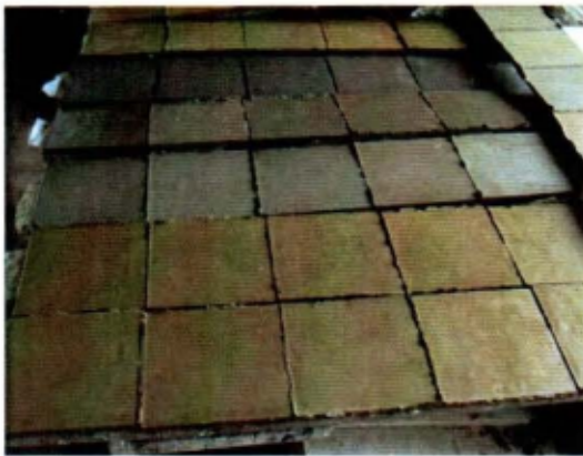
Plate XXX: Wet tiles produced by the researcher from Mukono clay, grog, kaolin and sand for decorating using embossed method.
