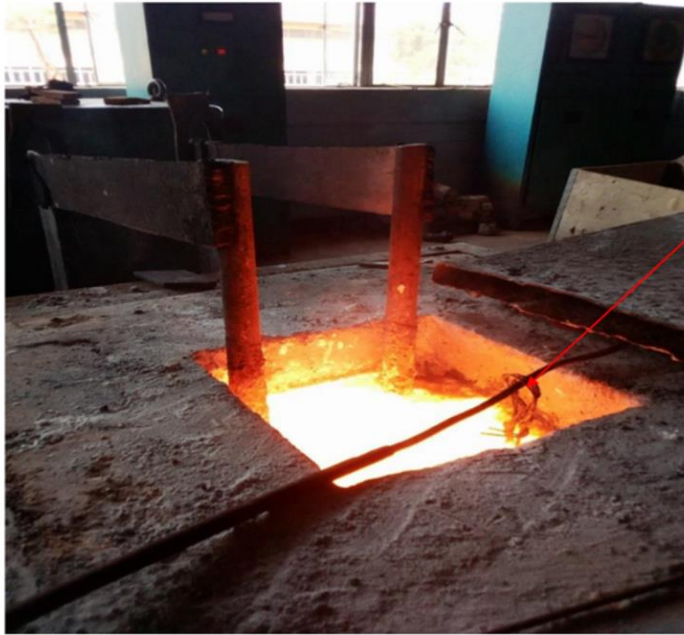
Figure 3. 10: Austenitizing the HSS tools in a single-phase salt bath resistance furnace (Longjiang Electric Furnace Works, 1989)
