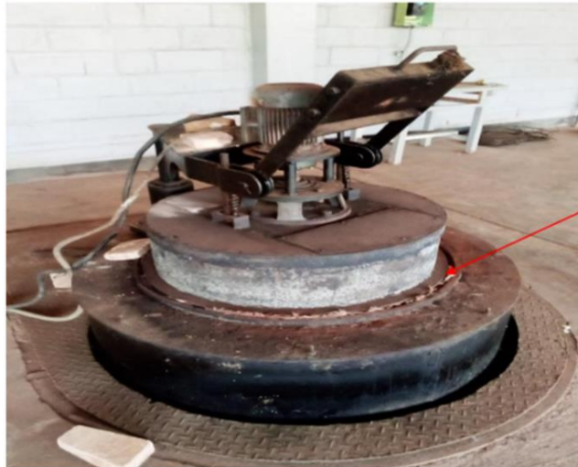
Figure 3. 12: Tempering the HSS tools in a pit well furnace
