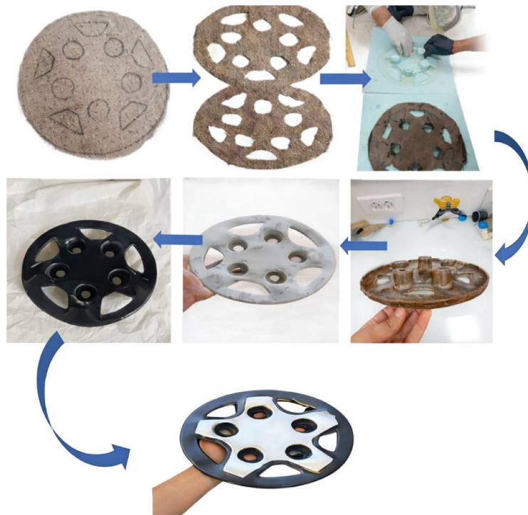
Figure 6. Compression moulding and final biocomposite hubcap after demoulding and finishing.
