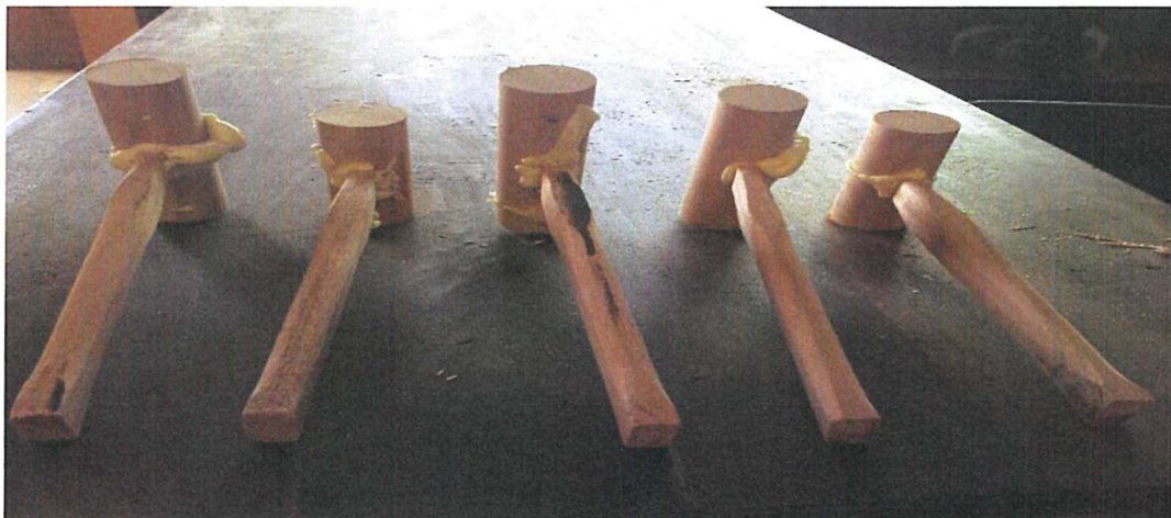
Figure 4. 6: Sample mallets done by students on the Lathe machine
