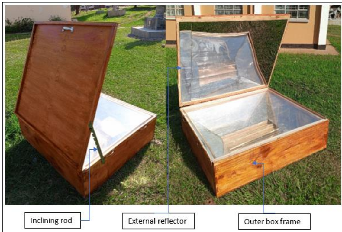
Figure 4.14: Full construction of the developed box-type solar cooker.
