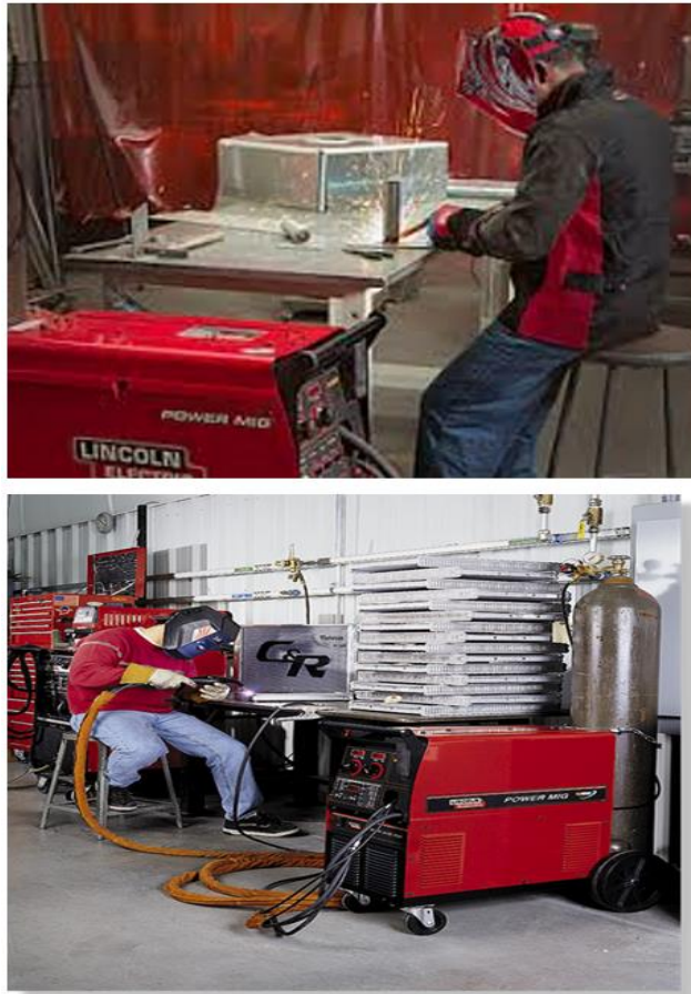
Figure 2-9: GMAW Process Welders in Action (Lincoln Electric, n.d.)
