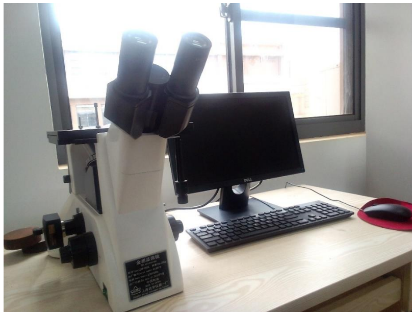
Figure F-2: Metallurgical Optical Microscope used for testing microstructural characteristics
