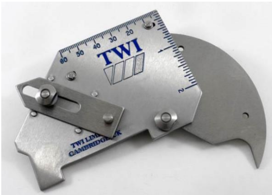
Figure A1-4: TWI Welding Gauge (Cambridge UK) (GAU/0002)
