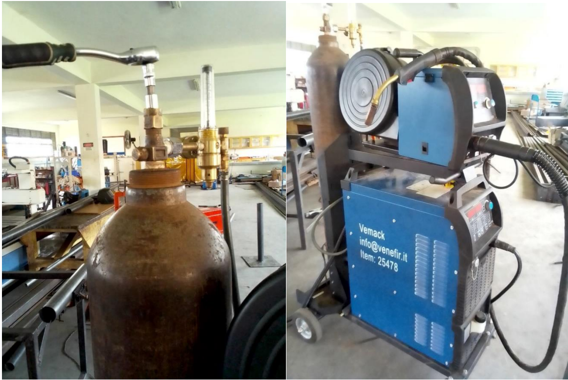
Figure A1-3: Shielding gas cylinder with gas control unit (left) and vermack GMAW welding set (right)
