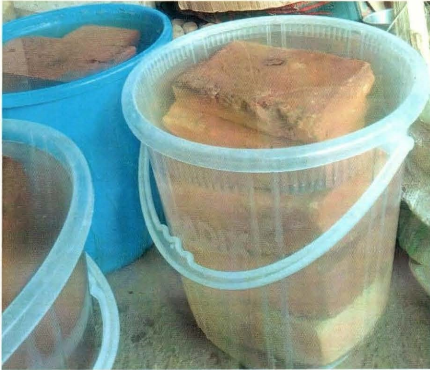
Figure 3.8: Total immersion of bricks in water
