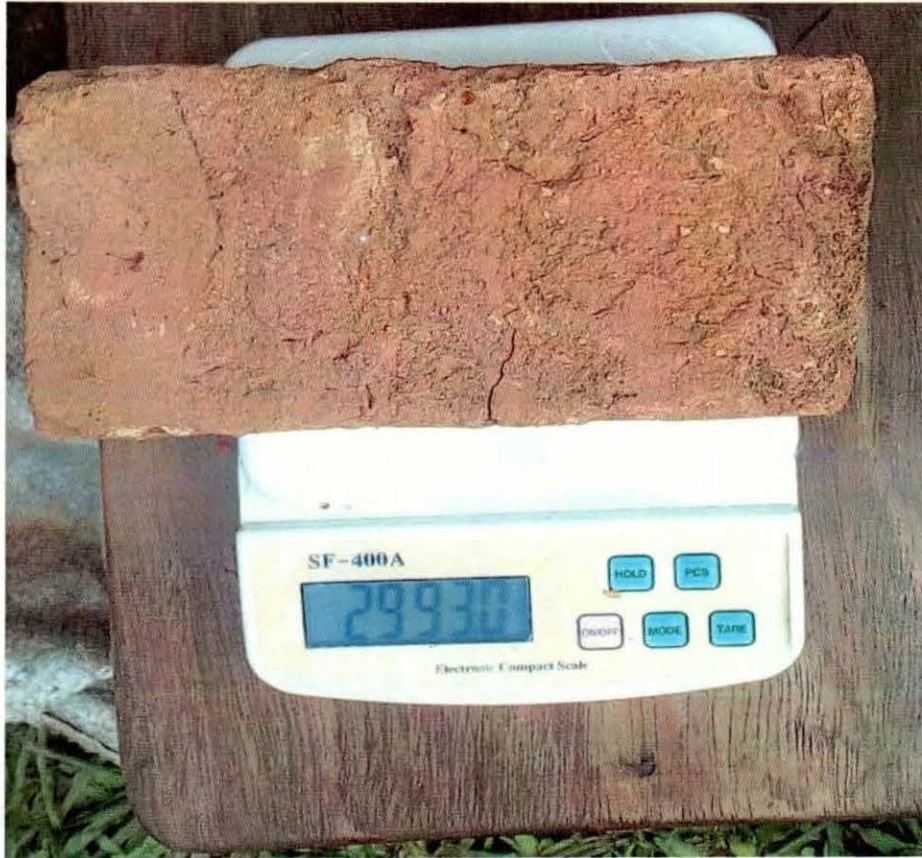
Figure 3.7: Dry brick being weighed
