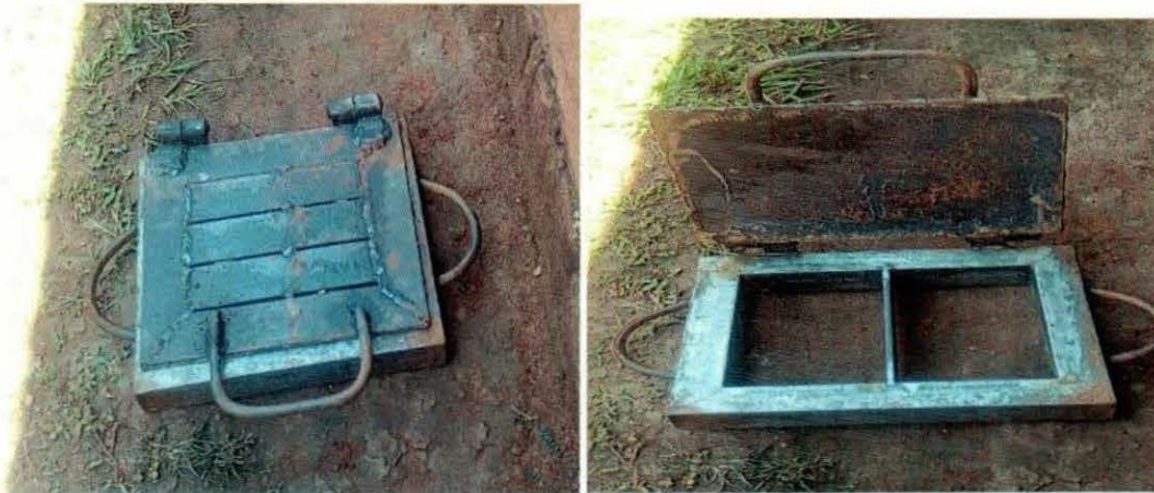
Figure 3.4: Improved metal mold due to its cover weight(10kg) that is used for uniform pressing of tempered clay during manufacturing
