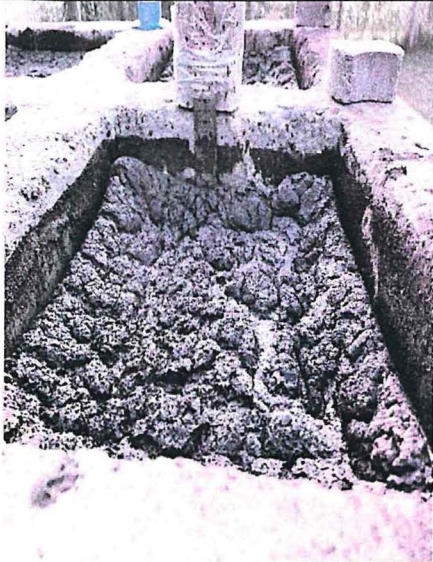
Shrinking solid sludge during dewatering
