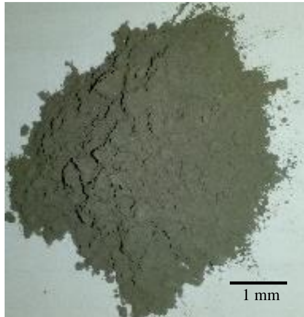
Figure 3. 2: The photo camera image of the as-received Bamburi Powerplus CEM I/42.5N.
