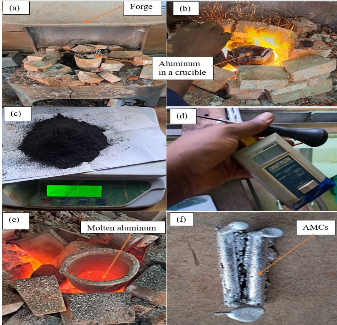
Figure 3.6: (a) The forging area, (b) Fire setup for melting aluminium, (c) The weighing scale, (d) The temperature gun, (e) Molten aluminium in the crucible and (f) Appearance of the fabricated AMCs before machining.
