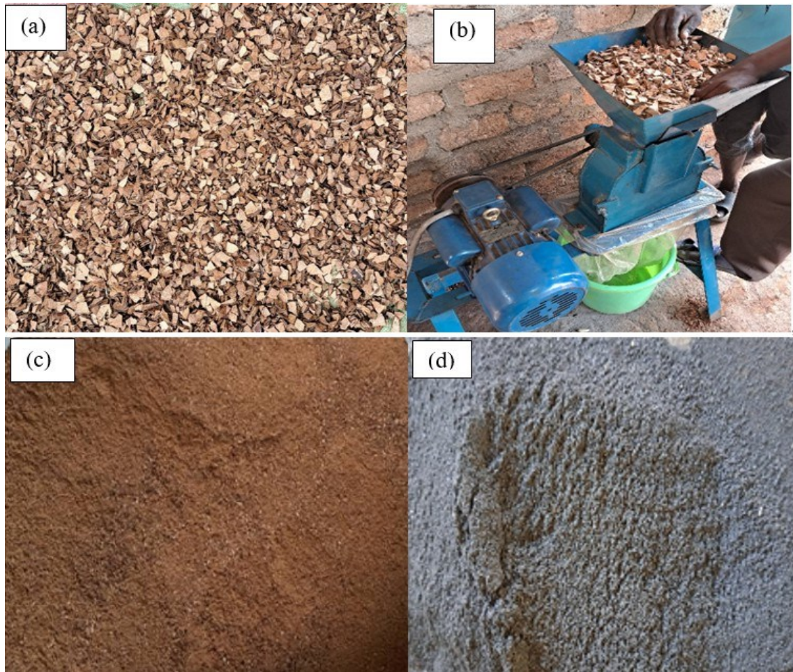
Figure 3.2: (a) Crushed coconut shells before milling, (b) Hammer milling process, (c) Coconut shell powder after milling and (d) Coconut shell ash after pyrolysis.
