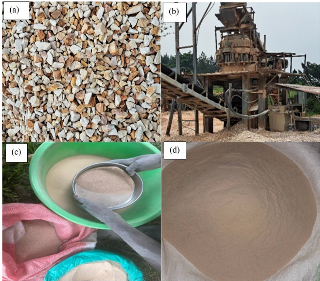
Figure 3.3: (a) Gravel, (b) Stone crushing machine, (c) The sieving process and (d) Fine crushed gravel powder.
