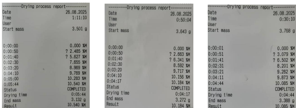
Fig.4.3: automatic print out of the amount of moisture content that was in the modified rice husk-based silica adsorbent.
