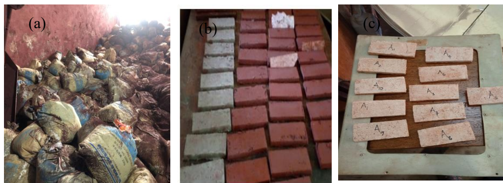
Figure A 2: (a) Ferric oxide waste at a steel factory, (b) green bodies after pressing, (c) sample tiles after firing.
