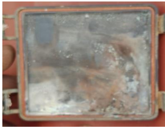
Figure 4.5: Diode cover corroded at Adwari Secondary School.
