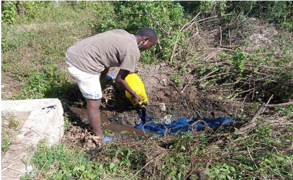
Figure 4.4: Mixing Brilliant Blue FCF in effluent at discharge.
