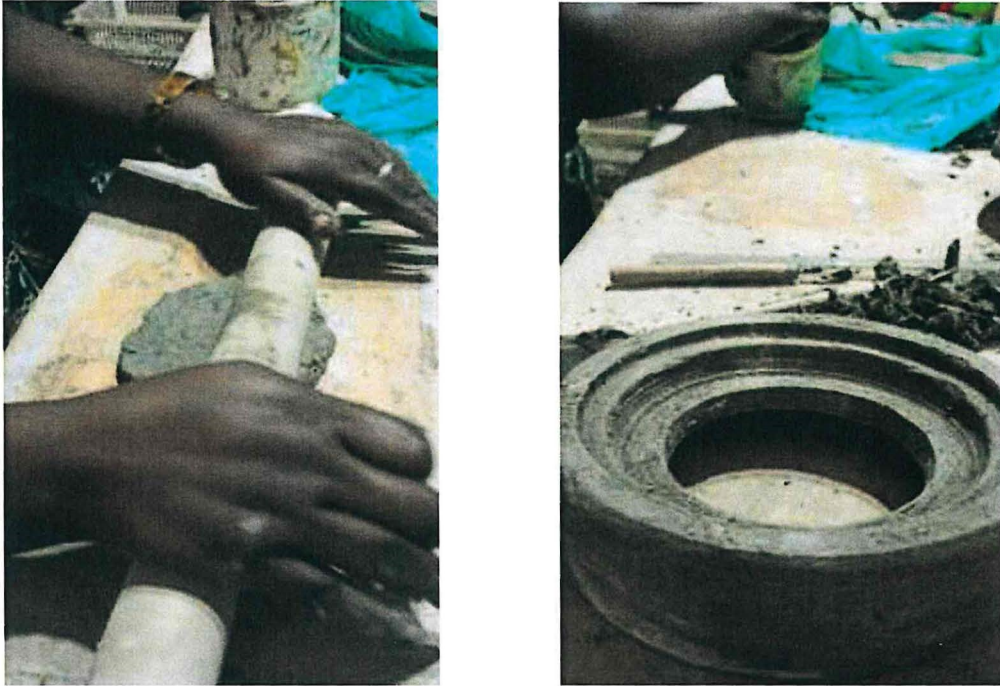
Figure 63: Rolling the slab to make the frame of the wall clock
