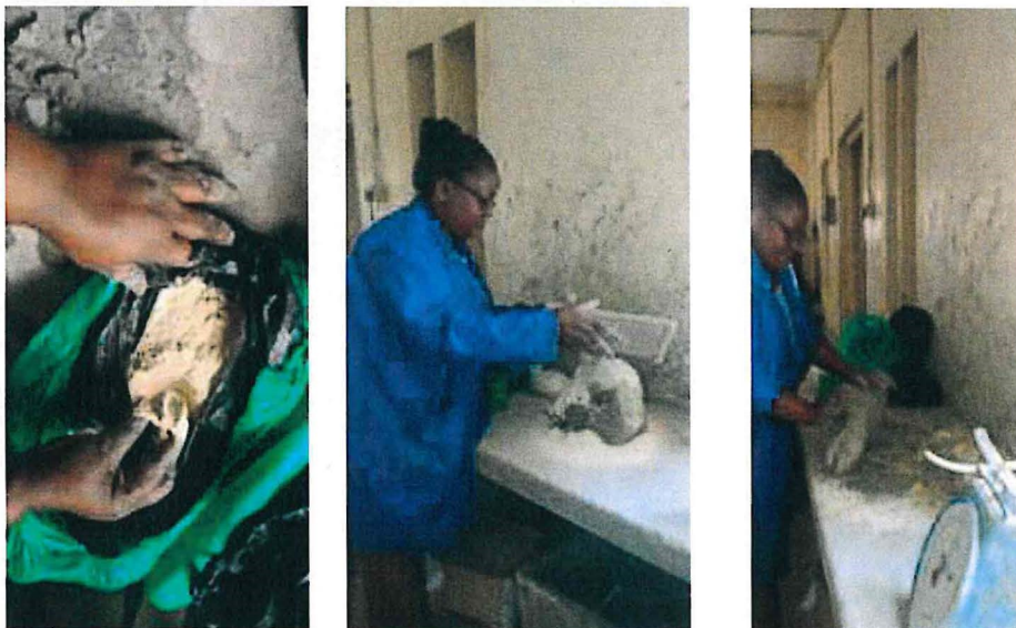
Figure 15: Wedging and kneading clay with Kaolin
