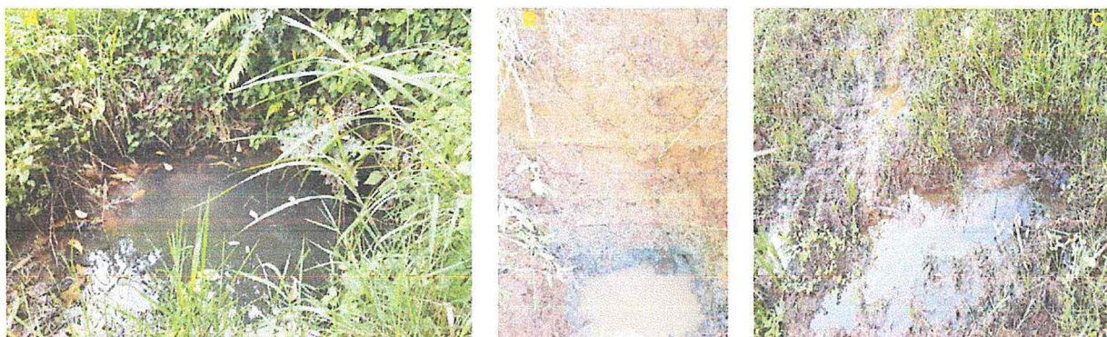
Plate 4.10: Seepage surfaces at selected landslide sites (A=Site 13LKN, B=Site 16MGS & C=Site 44CBZ)
