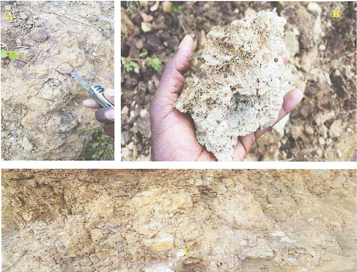
Plate 4.8: Strongly weathered bedrock material at selected landslide sites (A=site 45BZ, B= site 4BMS & C= site 35JBB)
