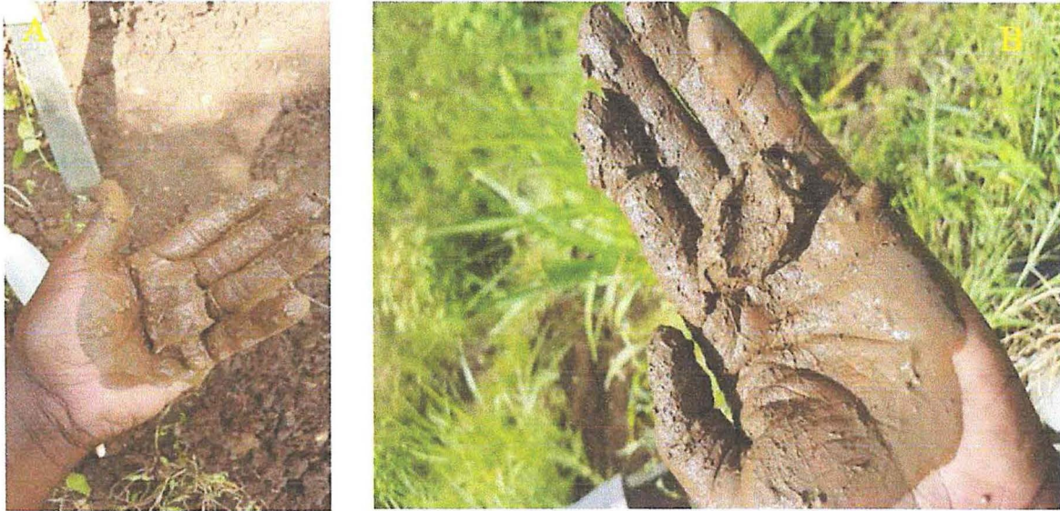
Plate 4.7: Testing for soil consistency at Zamalini (A) and Nakidibo (B) in Sisiyi sub-county
