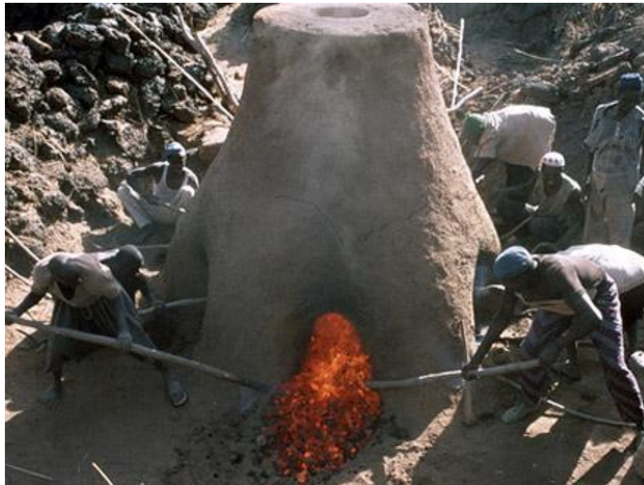
Figure 22: Furnace for indigenous Iron smelting in Mali
