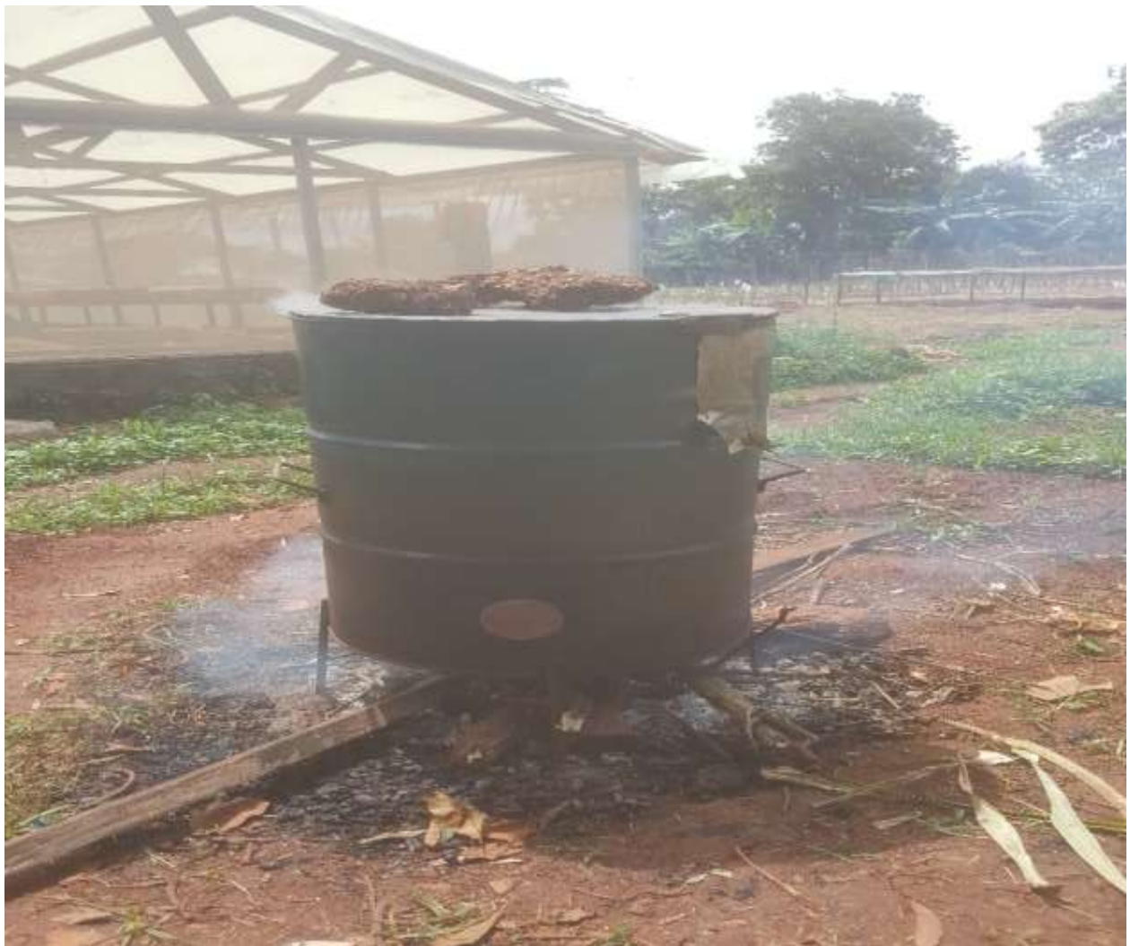
Plate 3: Sterilizing substrates by steaming at Kyambogo University, 2023-2024.
