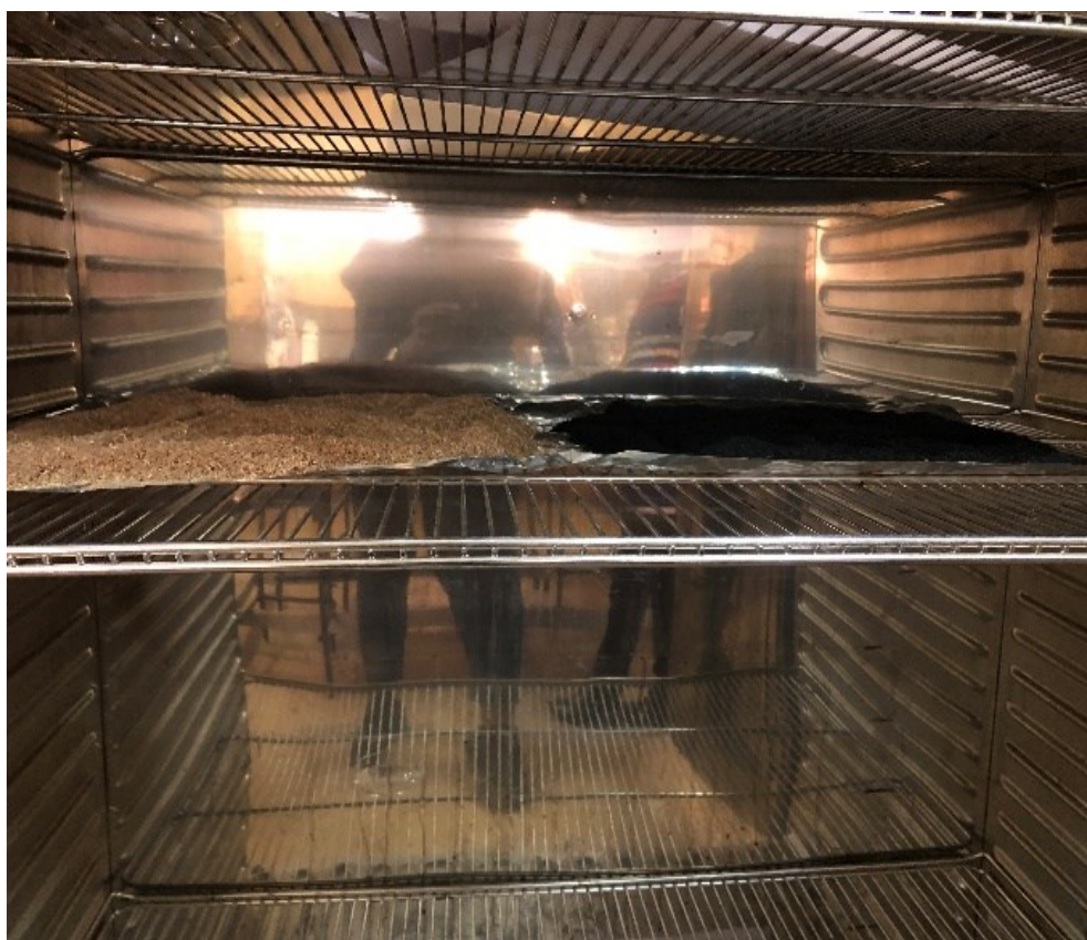
Figure 3.2: Placement of the sawdust and charcoal dust to be dried in the oven.
