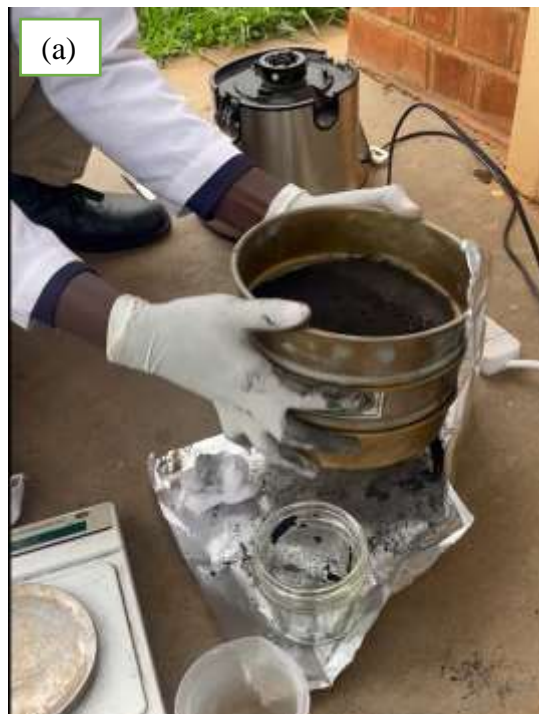
Figure 3.3: (a) Sieving of ground samples
