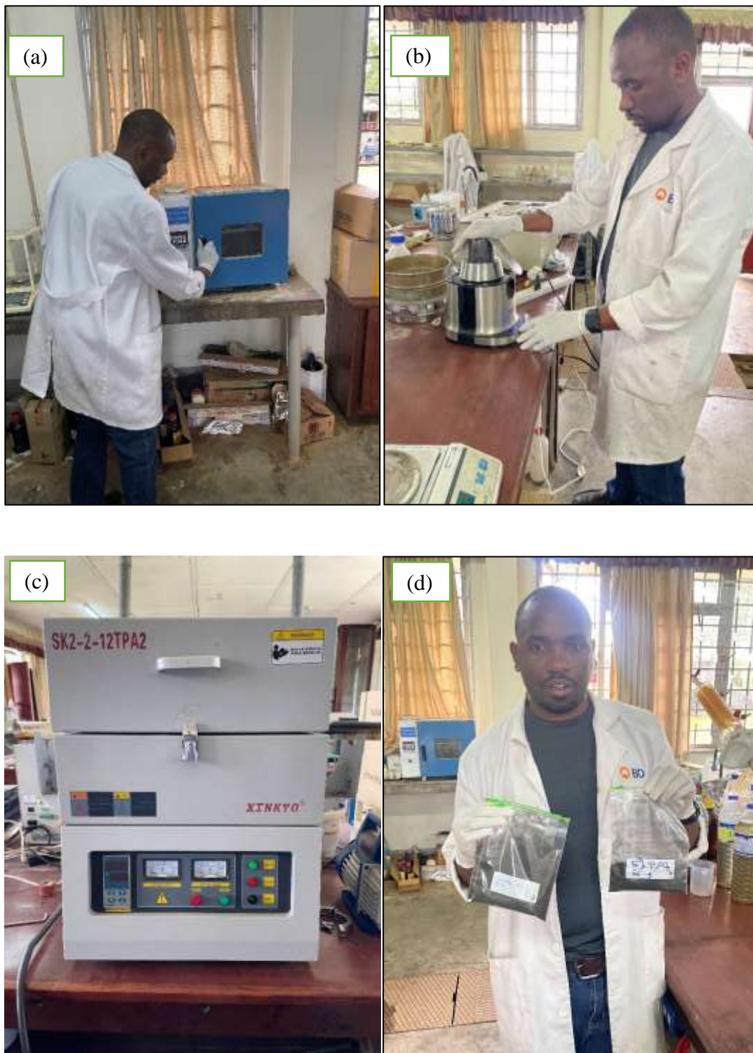
Figure 3.2: (a) Drying rice husk in an oven, (b) grinding rice husk in an electrical blender, (c) pyrolyzer used for carbonizing rice husk and (d) storing carbonized rice husk in air-tight clear cellulose bags.
