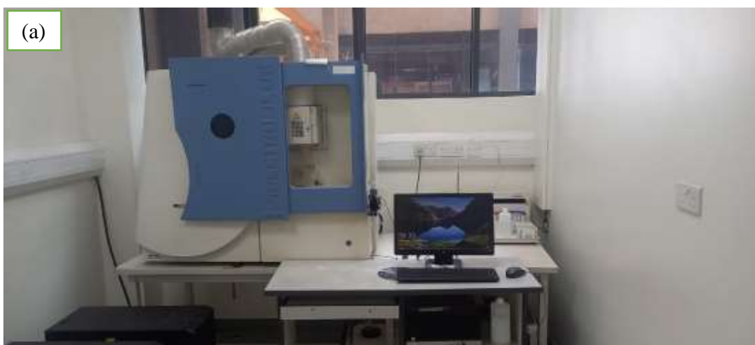
Figure 3.4: (a) The inductively coupled plasma-optical emission spectroscopy
