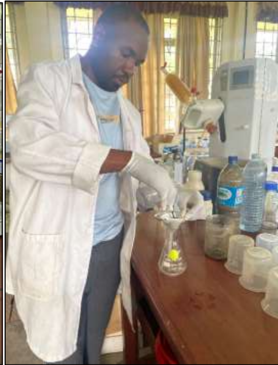
Filtering the solution of Pb^{2+} mixed with adsorbent
