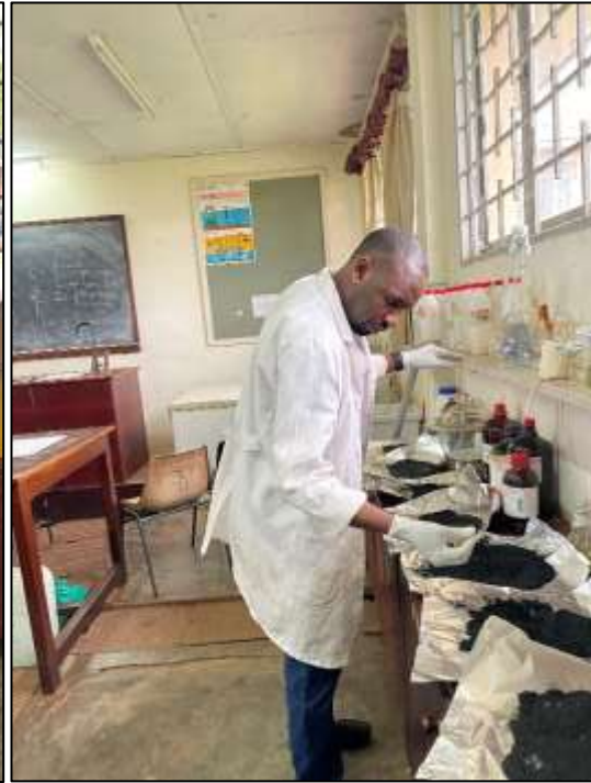
Checking on the RHC during drying
