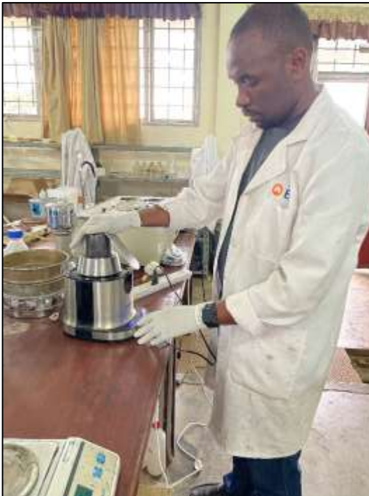
Grinding the RHC in blender
