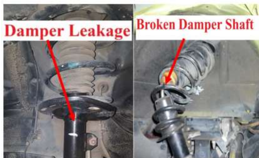
Figure 3. 1: A faulty Shock absorber with Fluid Leakages (Left) and a broken Shocker Absorber Piston after hitting pot hole. (Right)
