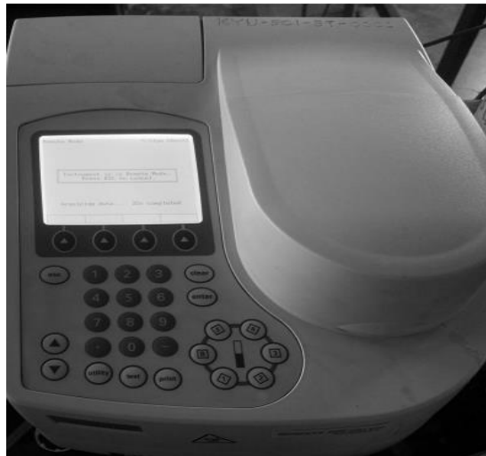
Figure 3.2: UV-Visible spectrophotometer (Photo was taken from the Chemistry laboratory of Kyambogo University)
