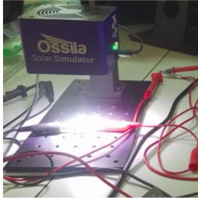
Figure 2.10: A solar simulator (Photo was obtained from the Physics laboratory of Kyambogo University)
