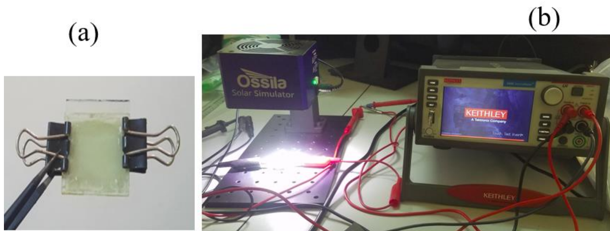
Figure 3.3: (a) Fabricated DSSC (b) Solar simulator and Keithley SMU-2450
