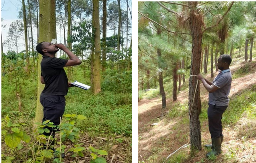
Plate A. 1: Measuring the tree height using a clinometer and diameter at breast height (DBH)
